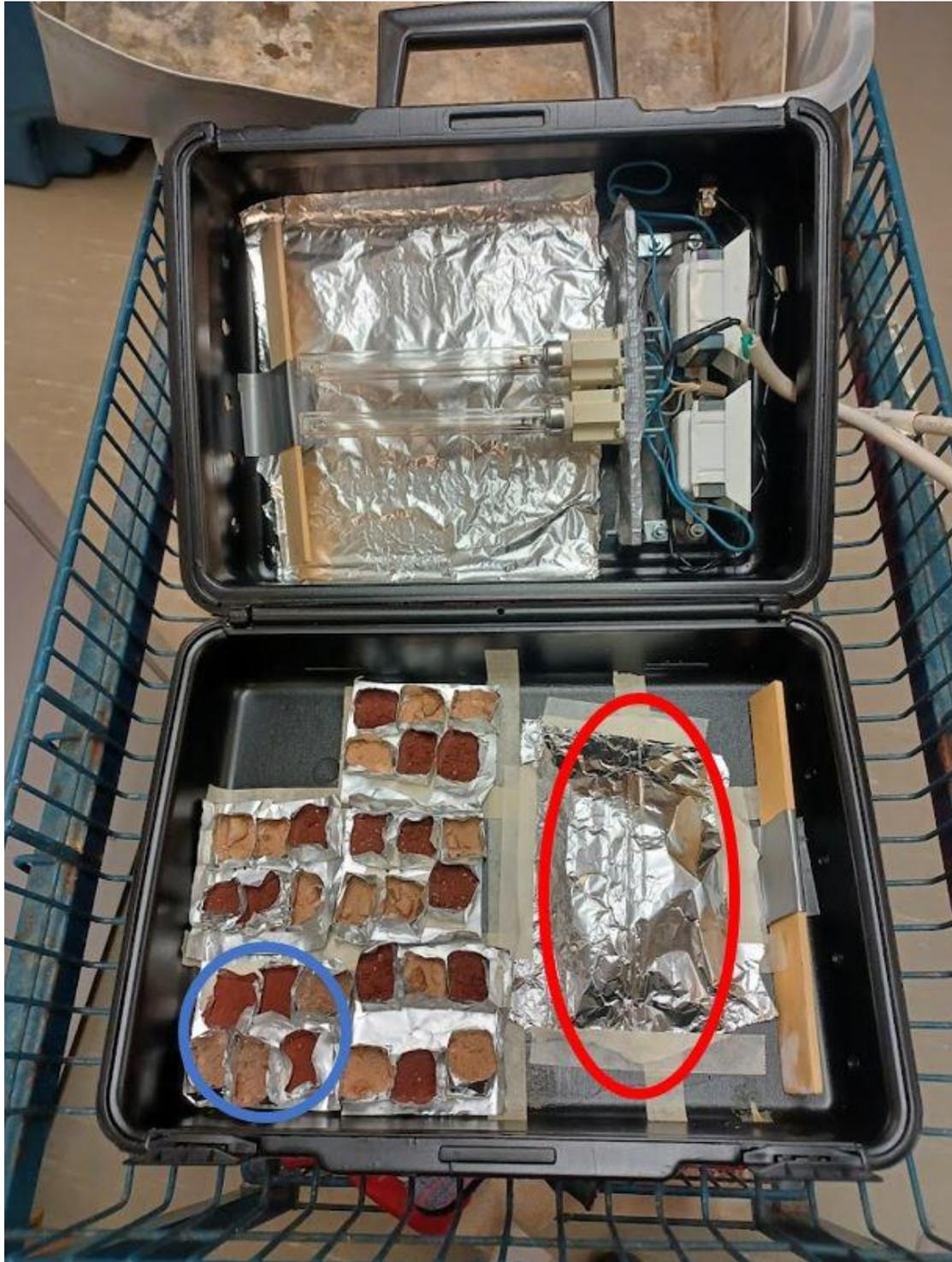
**Figure 3.3.** Custom UVC chamber containing University Valley cryptoendoliths. Unsterilized, covered negative control is circled in red. Sterilized and uncovered negative control is circled in blue.
