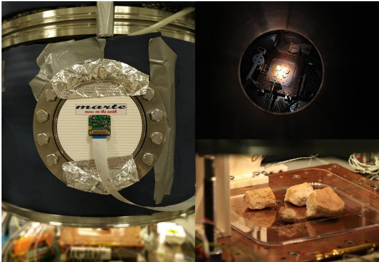
**Figure 3.2.** The MARTE vacuum chamber. Clockwise from left: MARTE exterior; interior and sample holder from MARTE's viewport containing University Valley cryptoendoliths; side view of University Valley cryptoendoliths in the MARTE sample holder.
