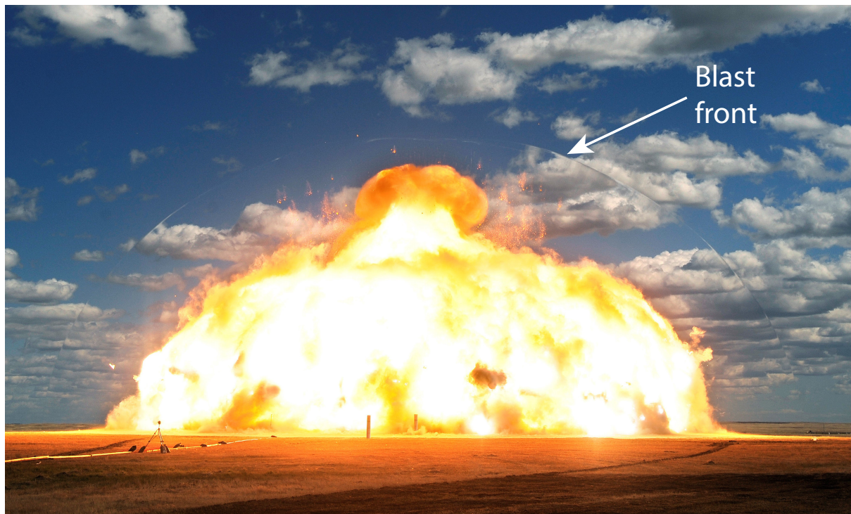
Fig. A.10 Fireball from the detonation of an explosively dispersed cloud of metal particles and fuel droplets. Photograph taken at DRDC Suffield, Alberta, Canada (cover picture of Shock Waves journal, Vol. 28, No. 3, 2018). The variation of the air refractive index due to the passage of the blast wave enables the visualization of the blast front.
