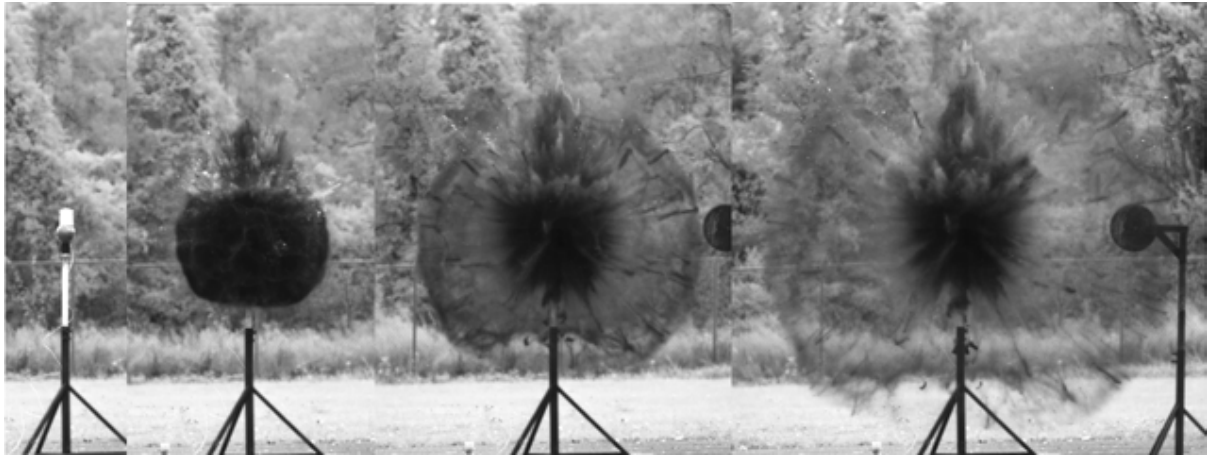
Fig. 2.3 Single video frames taken during the explosive dispersal of S110 steel shot. Charge diameter is 12.7 cm, mass of steel is 4130 g, mass of C-4 is 75 g, giving M/C = 55.1 . Pictures were taken 0, 2, 4, and 6 ms after detonation of the charge. Figure and caption courtesy of Loiseau et al. [17].
