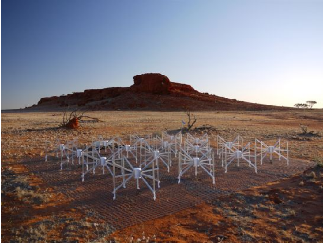
Figure 4–2: Photograph of an MWA antenna tile. 16 dual polarization 'bowtie' dipoles are arranged in a 4 \times 4 pattern. The wire mesh serves as a ground plane and also provides a reference grid to ensure each tile is laid out identically [20].
