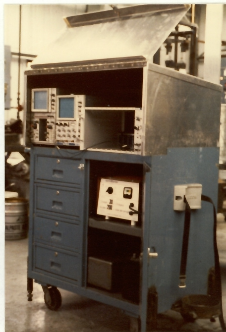
Figures 3 and 4: General view of the LiMCA apparatus as modified for carrying out in-plant trials.
