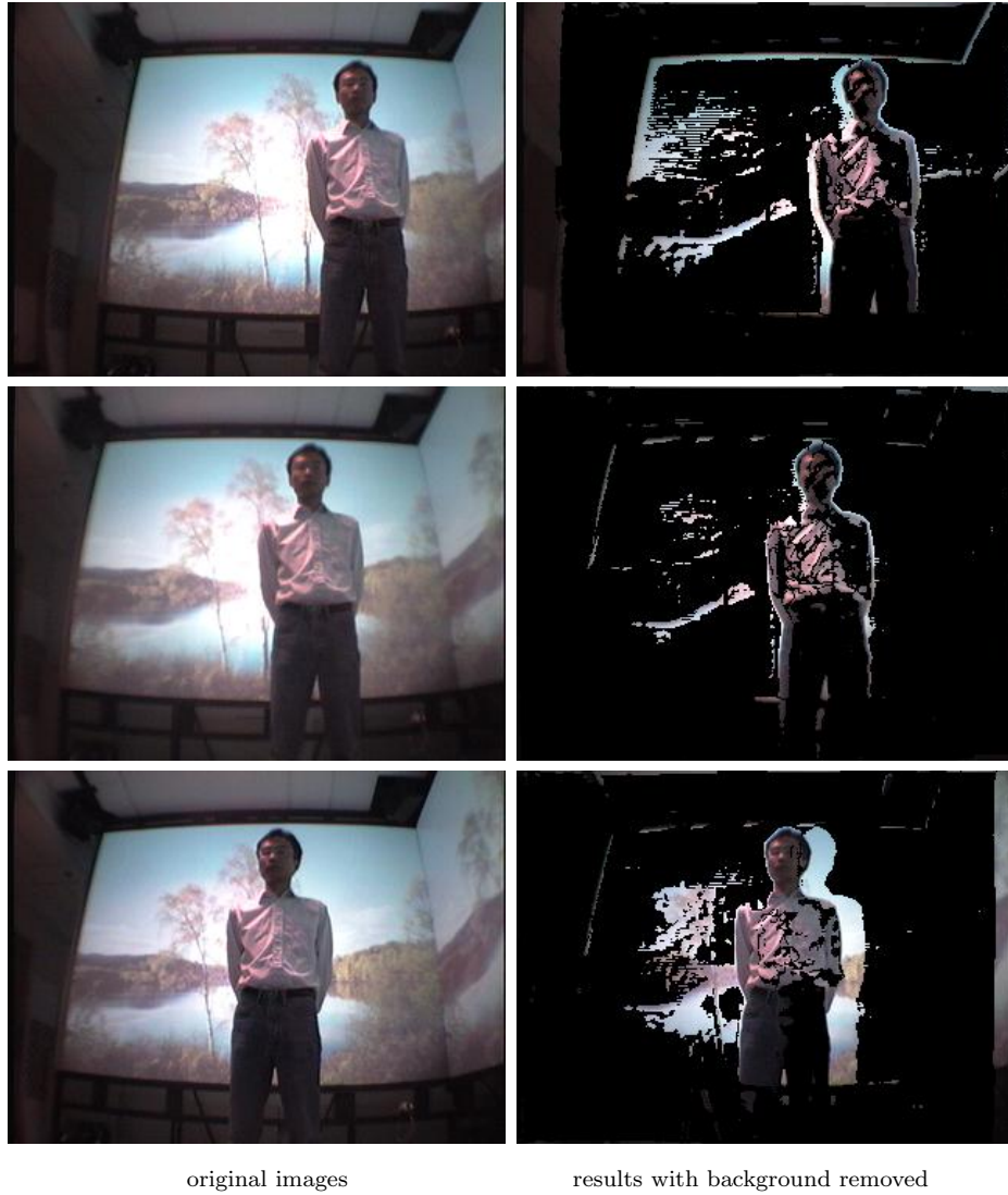
Figure 1-6: Background removal based on the known geometry. The planar screen (background) induces a homography transform between two cameras. If two pixels in two cameras related by the homography have the same color, they are regarded as projections of the same point (a background point) on the screen, and are removed. In the results, background pixels are painted as black.
