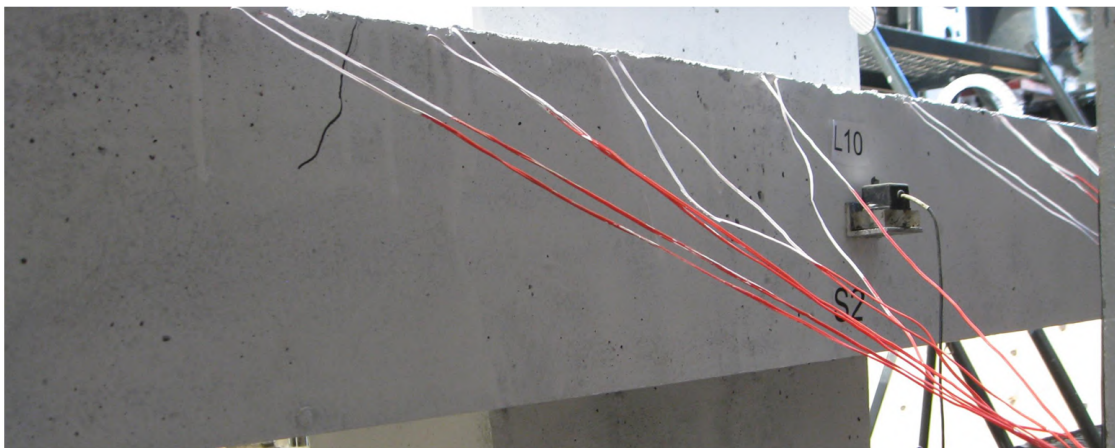
Figure 4.15: Specimen 2 free edge face cracks at V = 115.0 kN (west side)
