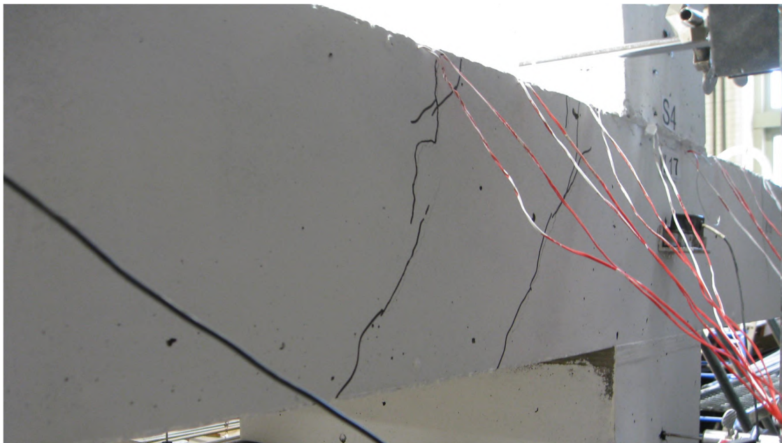
Figure 4.58: Specimen 4 free edge face cracks at V = 186.0 kN (east side)
