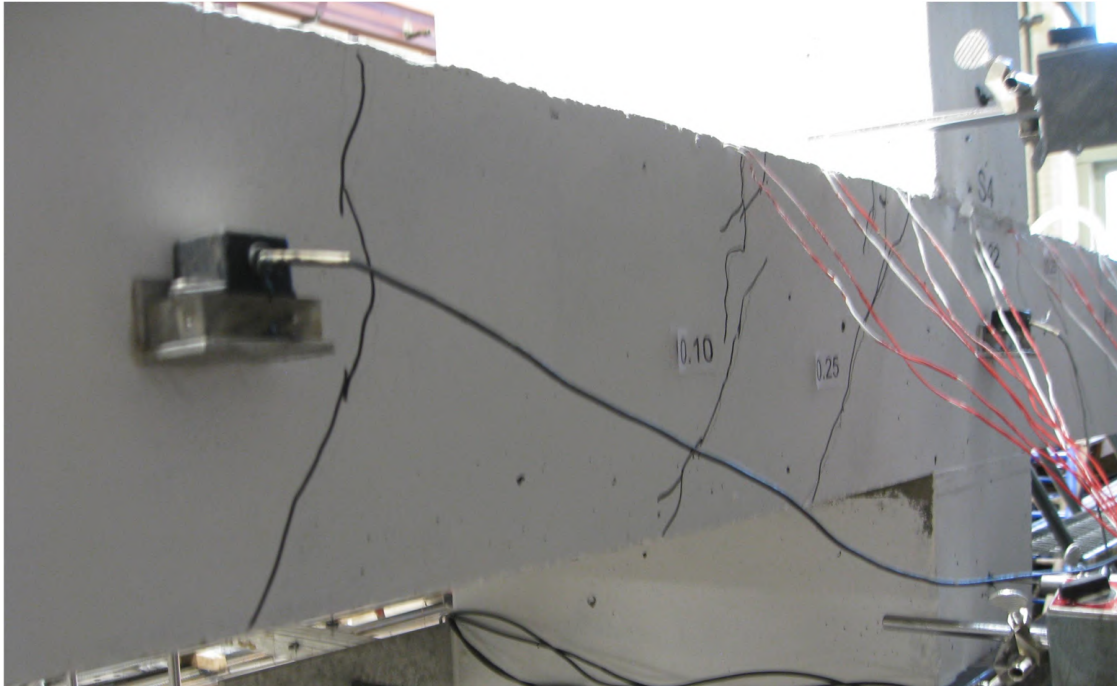
Figure 4.61: Specimen 4 free edge face cracks at V = 246.0 kN (east side)
