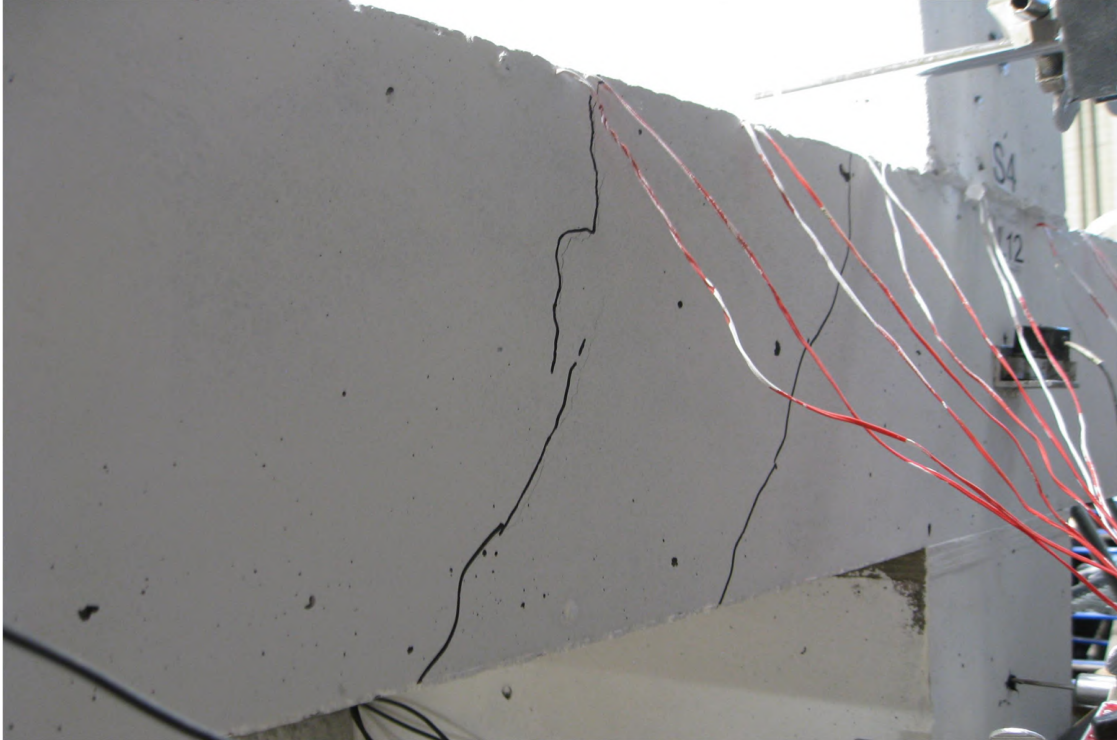
Figure 4.55: Specimen 4 free edge face cracks at V = 136.0 kN (east side)
