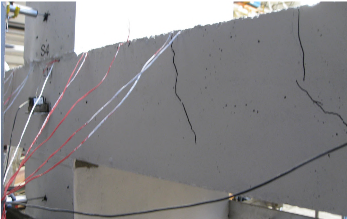
Figure 4.54: Specimen 4 free edge face cracks at V = 136.0 kN (west side)
