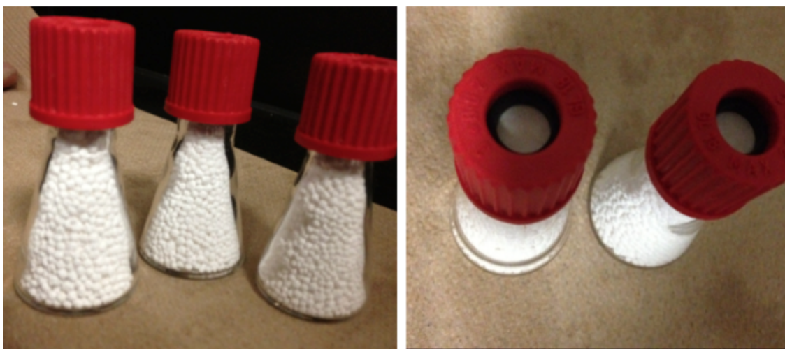
Figure 3.4. The assembled glass vials used for WVTR determination.
