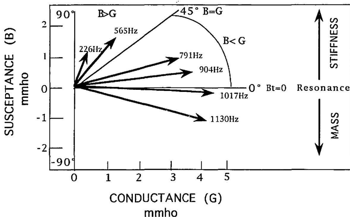
Figure 2. An example of admittance vector rotation as a function of frequency in a normal ear.
