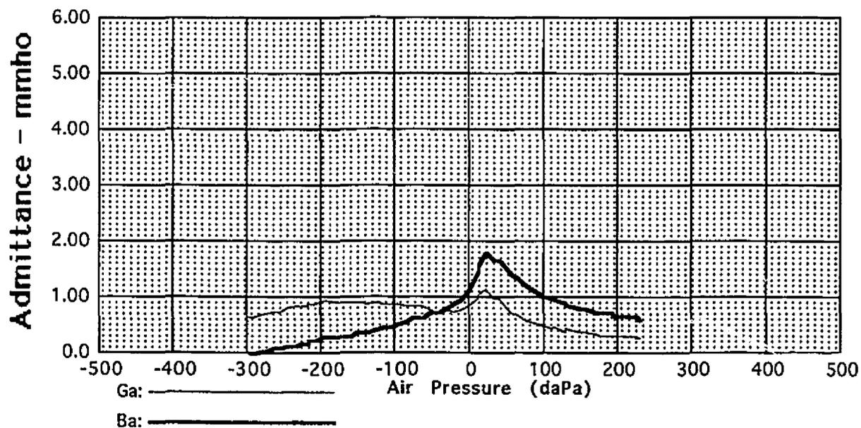
Figure 14. Admittance subcomponents at probe tone frequency of 450 Hz for the same subject as Figure 13.
