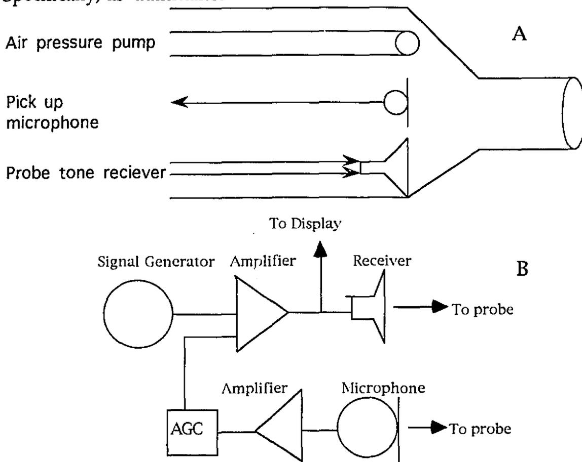
Figure 3. Block diagram of a probe assembly (A - top) and an admittance meter (B - bottom). (AGC = The automatic gain control).<sup>1</sup>
