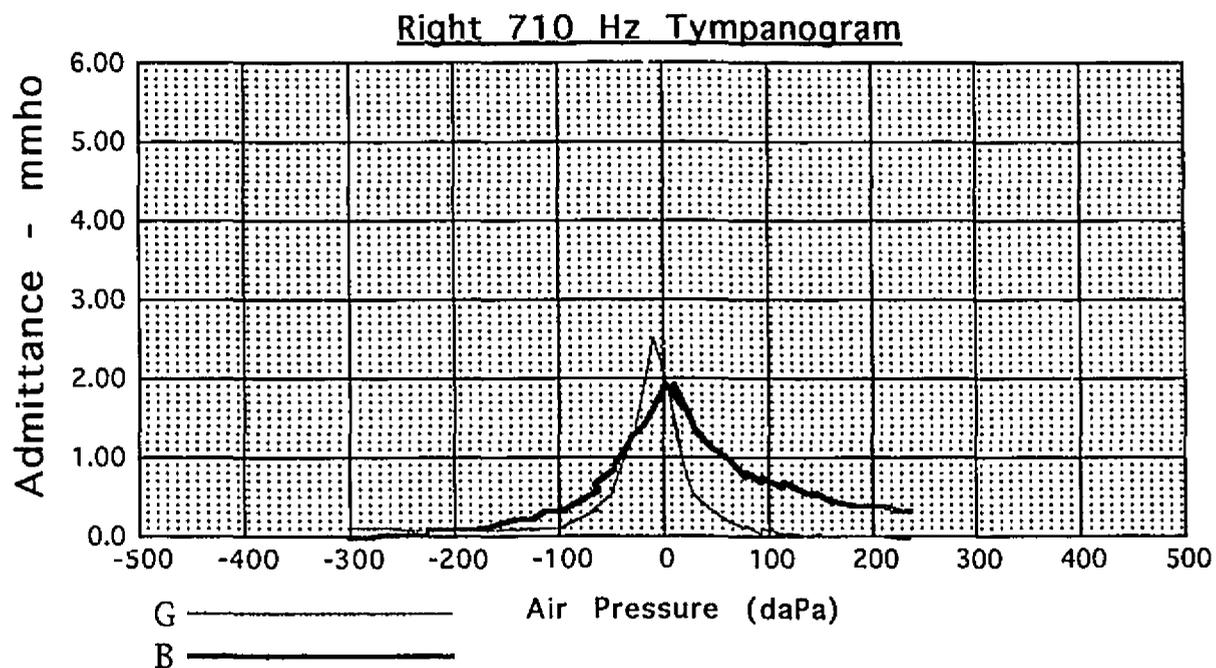
Figure 21. Illustration of the method used to estimate the admittance phase angle of  $45^\circ$ . In this example the frequency at which conductance(G) first became larger than susceptance(B) was 710 Hz.
