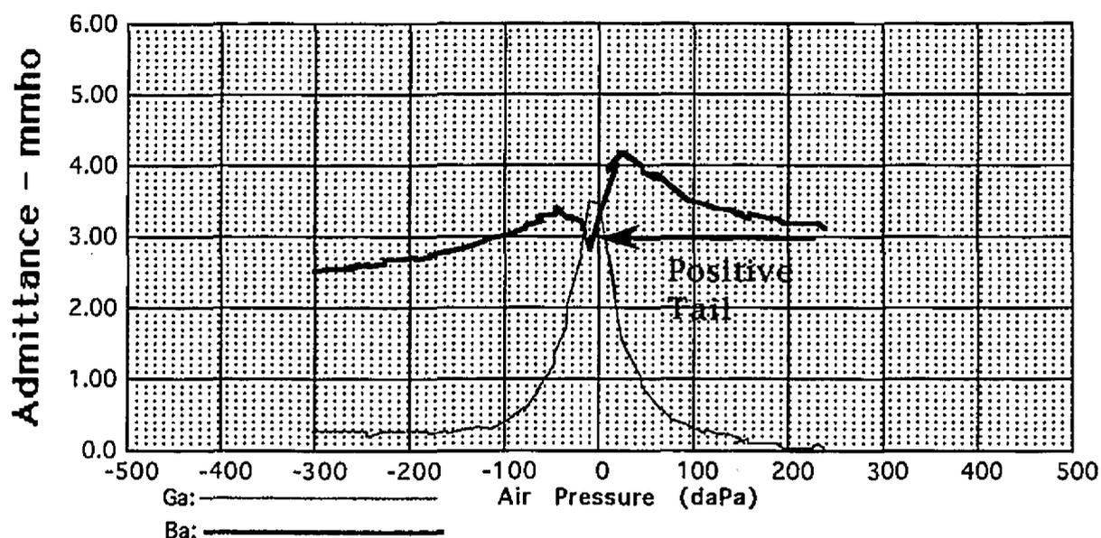
Figure 15. Illustration of a susceptance (B) tympanogram near the resonant frequency when positive tail compensation is used. Resonant frequency corresponds to the lowest frequency ( 900 Hz in this example) at which the central notch in the susceptance (B) tympanogram falls at or below the positive tail.
