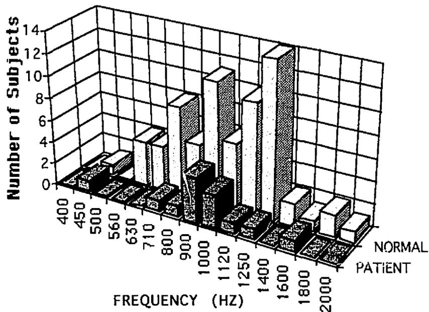
Figure 11. Distribution of resonant frequencies estimated by the screening mode for normal and otosclerotic ears.
