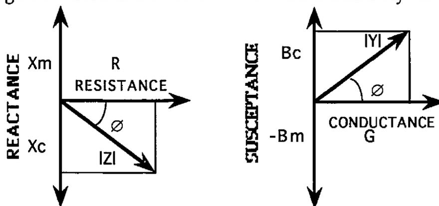
Figure 1. Left - The impedance vector [ $X_m$ : mass reactance;  $X_c$ : stiffness reactance;  $|Z|$ : absolute impedance magnitude;  $\phi_z$ : impedance phase angle]. Right - The admittance vector [ $B_m$ : mass susceptance;  $B_c$ : stiffness susceptance;  $|Y|$ : absolute admittance magnitude;  $\phi_y$ : admittance phase angle].
