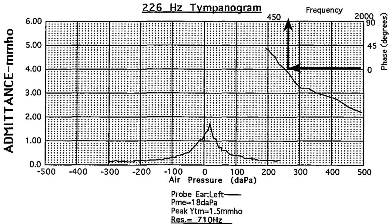
Figure 10. Illustration of data provided by resonance screening. The  $\theta_{tm}$  is plotted as a function of the probe tone frequency from 500-2000 Hz in the upper right corner of the display. Resonance is derived as the frequency corresponding to a phase angle of zero° on this function, (710 Hz in this example).
