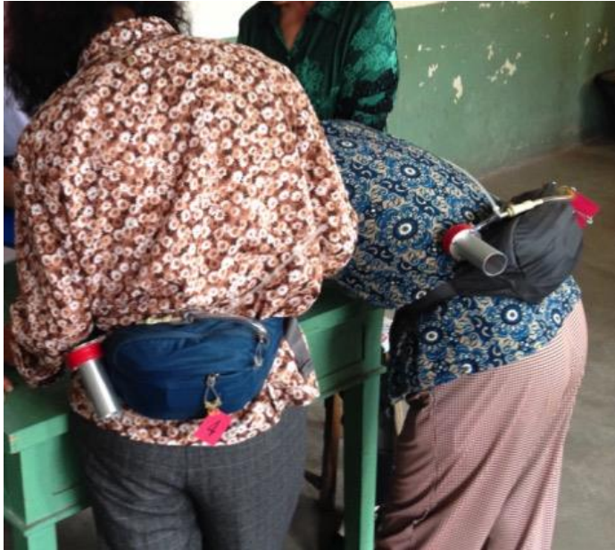
Figure S2: Setup of the Harvard Personal Exposure Monitor within waistpacks (Photo credit: Ellison Carter)
