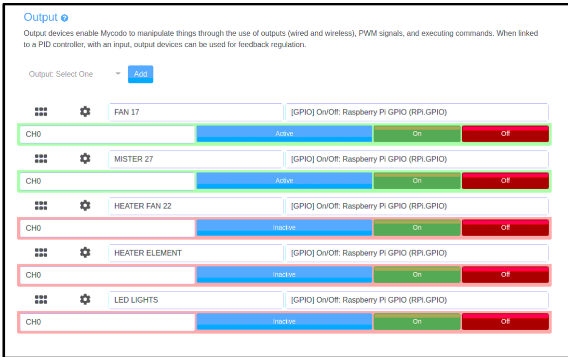
Figure 19: Output configuration of the electric components
