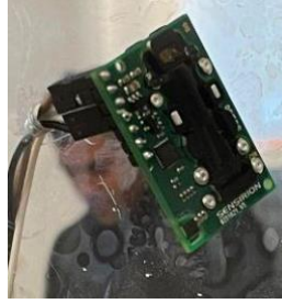
Figure 9: SCD30 sensor, for the monitoring of temperature, relative humidity, and CO 2 levels
