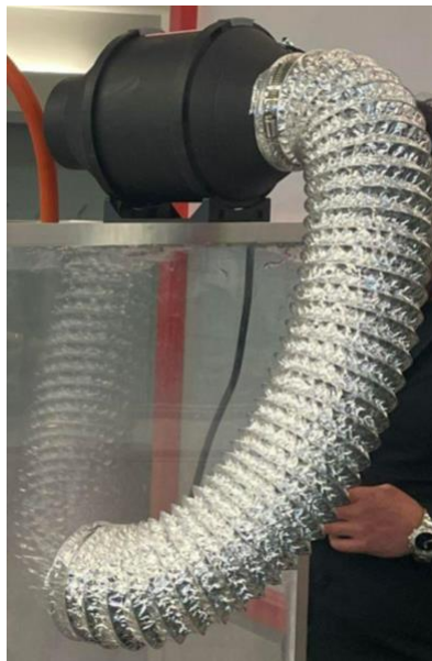
Figure 15: Exhaust fan, used for expelling CO 2
