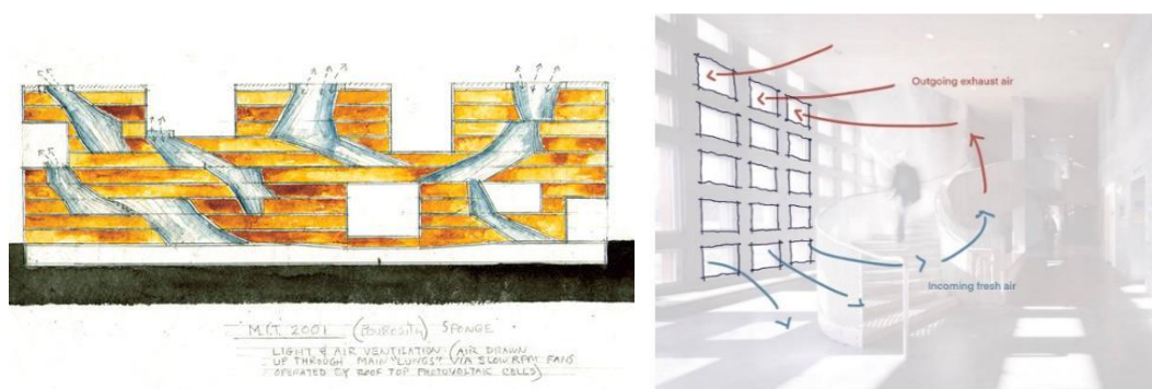
Figure 4.8: Diagrams of two means of natural ventilation in Simmons Hall
