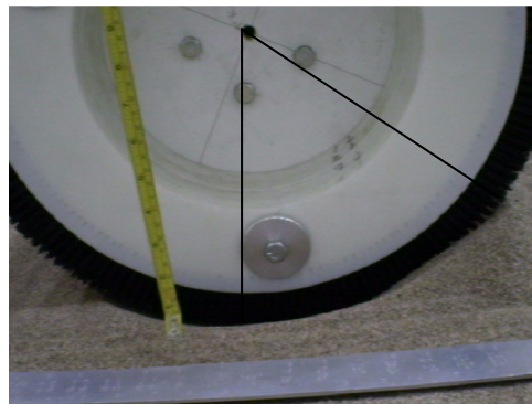
Brush wheel (534 N load) 100% slip \theta_2 = -57.5^\circ
