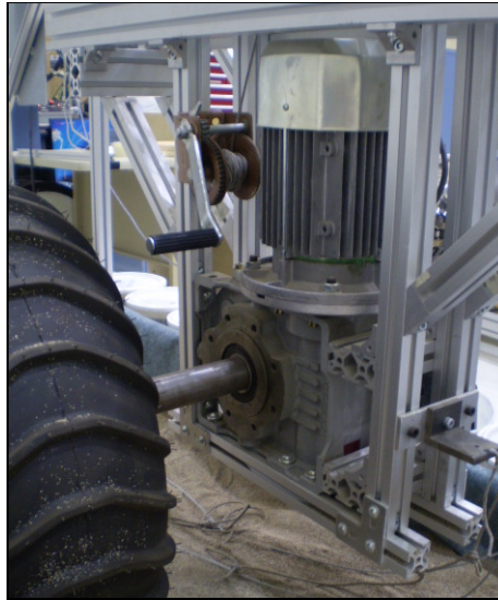
Fig. 3.6: Single wheel testbed: motor and gear box assembly
