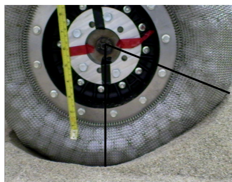
iRing wheel (500 N load) 100% slip \theta_2 = -67.1
