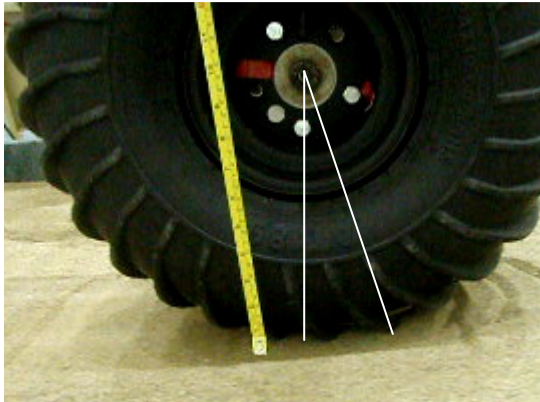
d) Rubber wheel (373 N load) 2.5 psi (no slip) \theta_2 = -25.9
