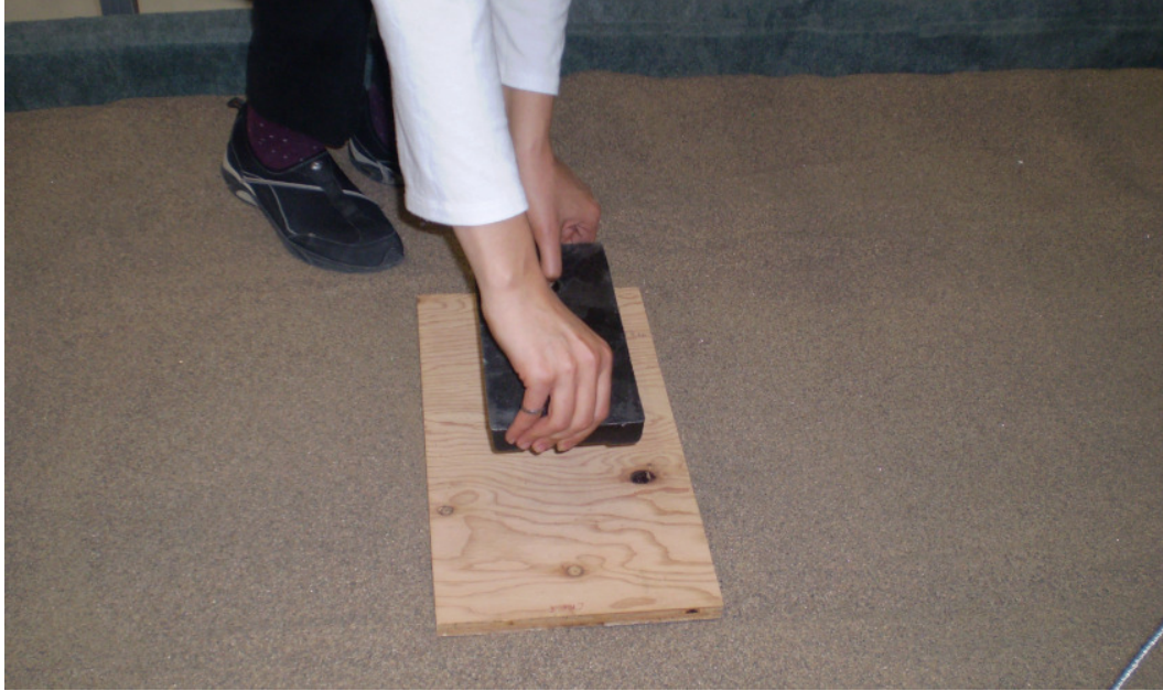
Fig. 3. 16: Preparation of the soil surface prior to wheel testing
