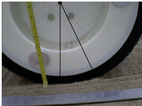
a) Brush wheel (534 N load) No slip \theta_2 = -26.5^\circ
