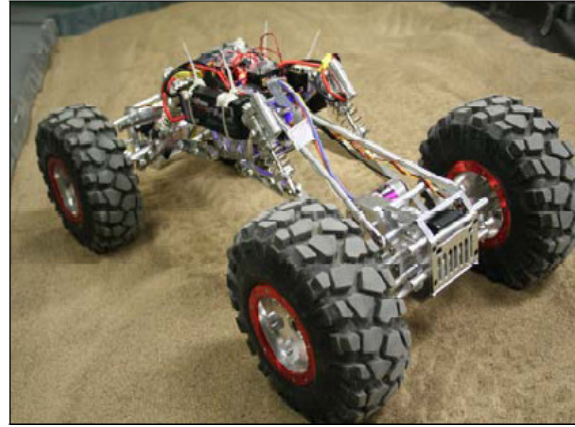
b) Testbed for 8" diameter wheels
