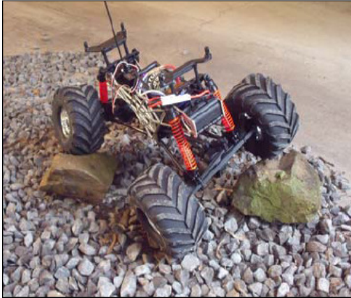
a) Testbed for 5" diameter wheels
