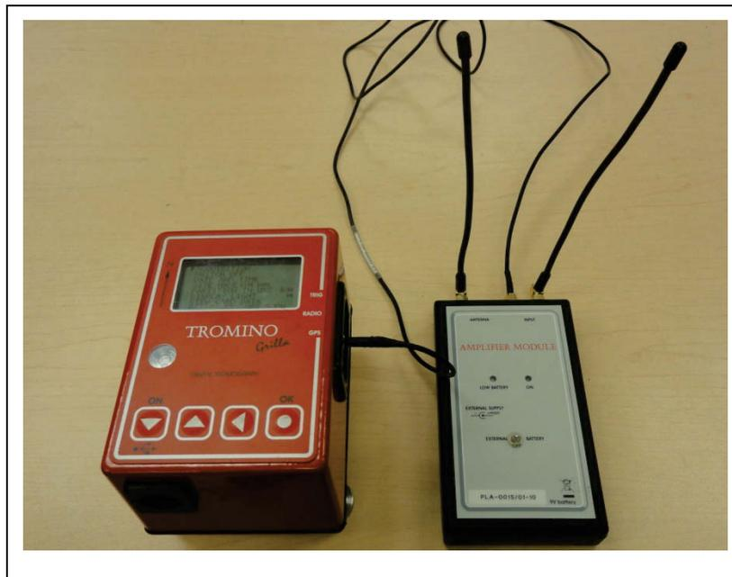
**Figure 12 - TROMINO sensor connected to the radio antenna**
