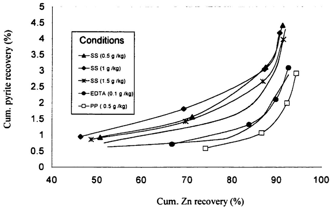
Fig. 4.24 Cumulative pyrite recovery vs Zn recovery for various conditions. Note: Pyrite grade was computed from the metal assays allowing for Fe in chalcopyrite and 6.6 % Fe in sphalerite.
