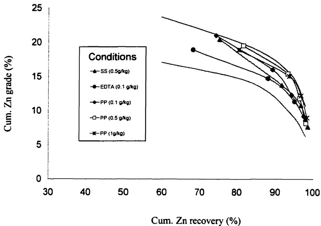
Fig. 4.28 Cumulative Zn grade vs recovery for various conditions.
