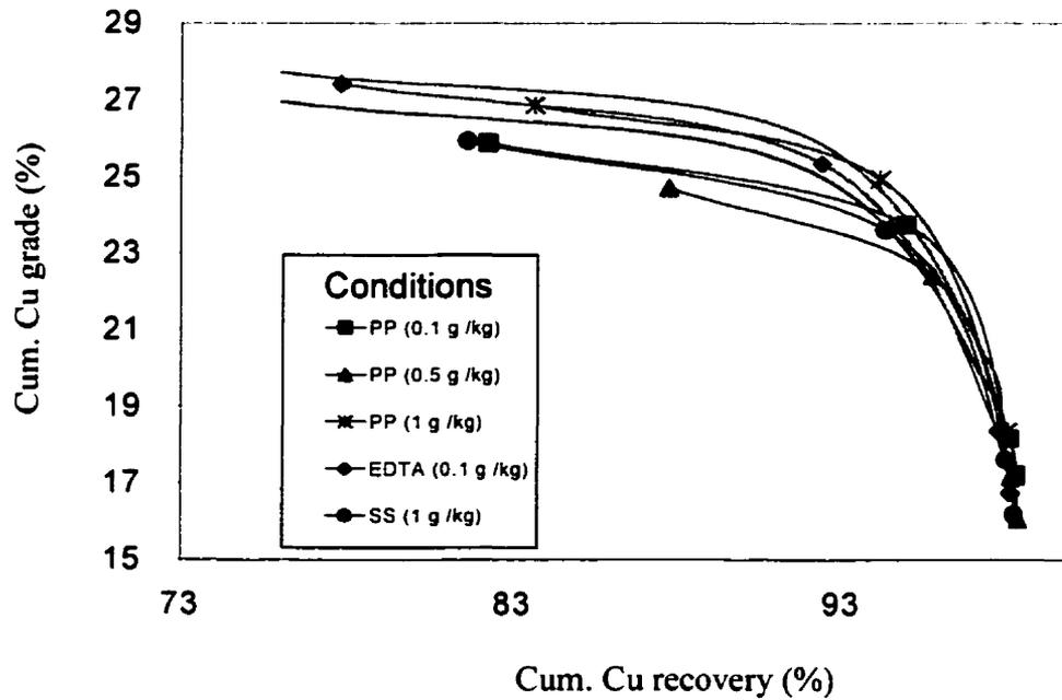
Fig. 4.21 Cumulative Cu grade vs recovery for various conditions.
