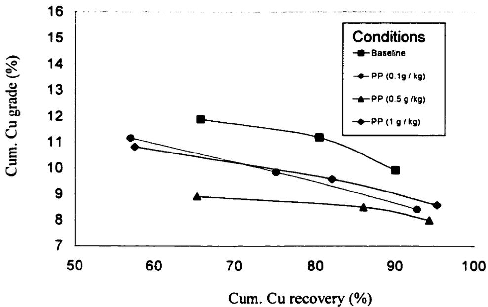
Fig. 4.25 Cumulative Cu grade vs recovery for various concentrations of polyphosphate.
