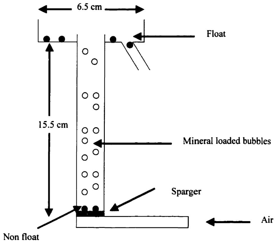
Fig. 3.1 Micro flotation set-up
