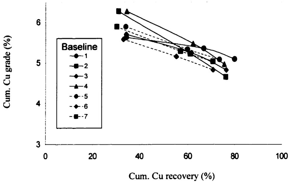
Fig. 4.15a Repeatability: Baseline cumulative Cu grade vs recovery test results - Les Mines Selbaie with NaCN added in grinding.
