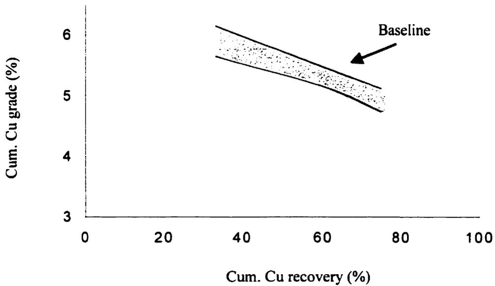
Fig. 4.15b 95 % confidence interval band derived from Fig. 4.15a.
