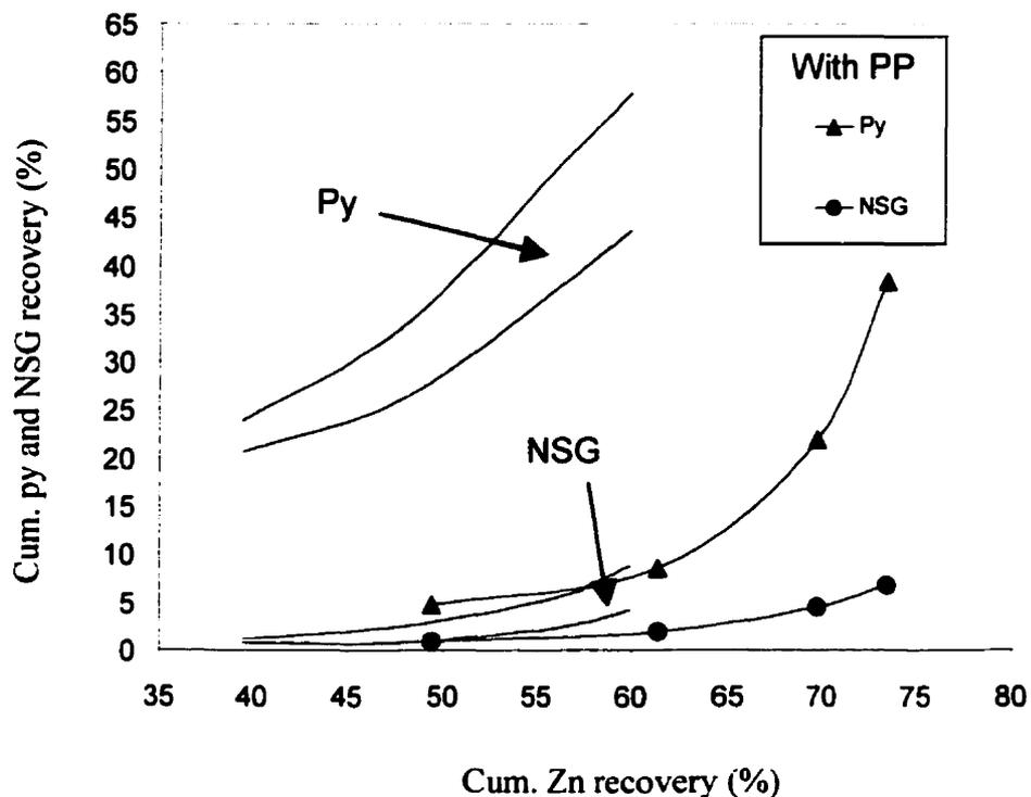
Fig. 5.3 Cumulative pyrite and non sulphide gangue recovery vs Zn recovery for Les Mines Selbaie (baseline - shaded area, and with 0.5 g /kg PP - symbols).
