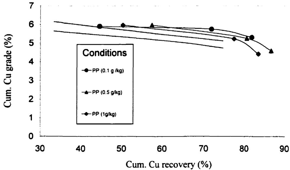
Fig. 4.18 Cumulative Cu grade vs recovery for various concentrations of polyphosphate with NaCN.
