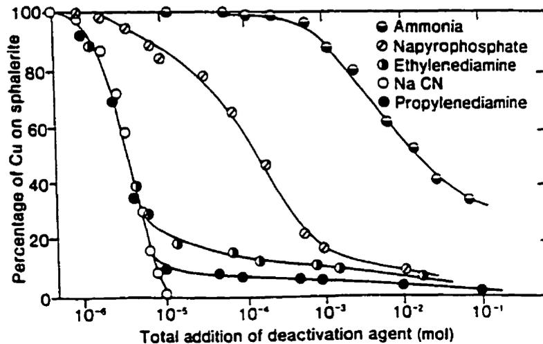
Fig. 2.5 Partition of copper between solution and sphalerite as a function of the addition of deactivating agent (after: Gaudin et al., 1959).
