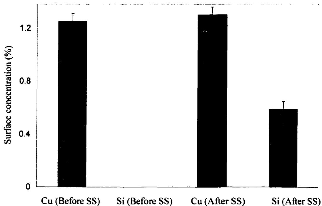
Fig. 4.12 Surface concentration of Cu and Si on Cu activated pyrite surface before and after silica sol (SS) addition at pH 9. Note: Error bar is  $2\sigma$ .
