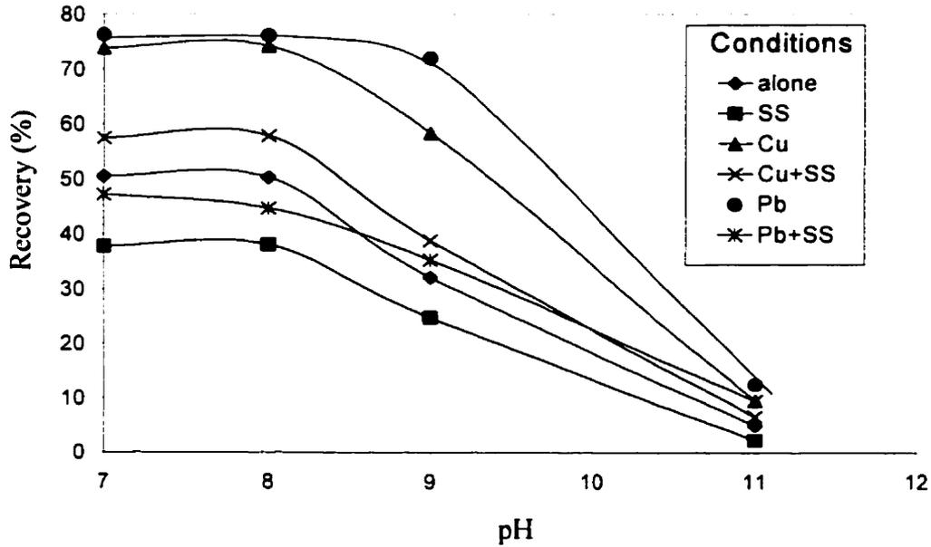
Fig. 4.6 Oxidized pyrite recovery as function of pH for various conditions.
