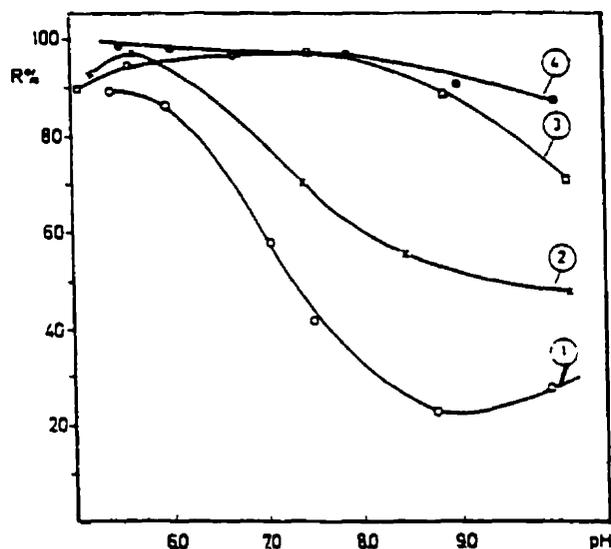
Fig. 2.3 Flotation recovery of sphalerite as a function of pH: 1= without reagents; 2 =  $3.1 \times 10^{-5}$ ; 3 =  $6.2 \times 10^{-5}$ ; 4 =  $1.5 \times 10^{-4}$  mol dm<sup>-3</sup> KEX (after: Popov et al., 1989).
