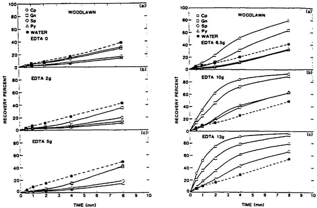
Fig. 5.1 Influence of EDTA on flotation of sulphides from Woodlawn ore
