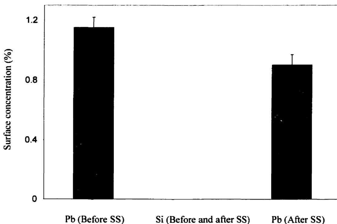
Fig. 4.10 Surface concentration of Pb on Pb activated sphalerite surface before and after silica sol (SS) addition at pH 9. Note: Error bar is  $2\sigma$ .
