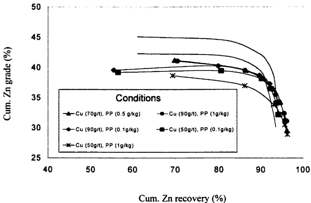
Fig. 4.31 Cumulative Zn grade vs recovery for various combinations of  $\text{CuSO}_4$  and polyphosphate: PP added prior to  $\text{CuSO}_4$ .
