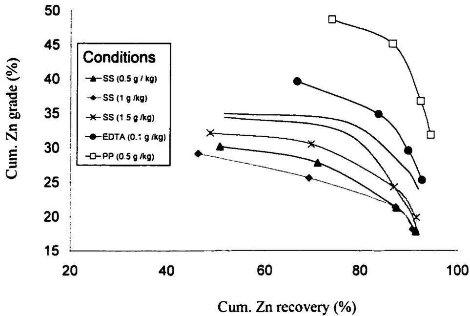
Fig. 4.23 Cumulative Zn grade vs recovery for various conditions.
