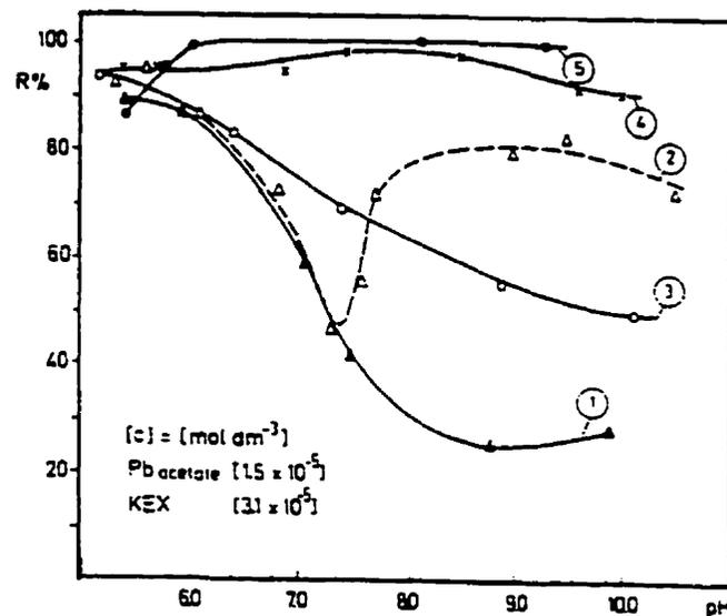
Fig. 2.4 Flotation recovery of sphalerite as a function of pH: 1 = no reagents; 2 = Pb acetate; 3 = KEX; 4 = Pb acetate (pH 5 - 6) and KEX; 5 = Pb acetate and KEX, 8 < pH activation = pH flotation < 9 (after: Popov et al., 1989).
