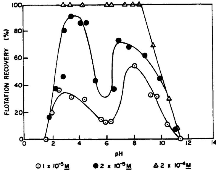
Fig. 2.6 Recovery of pyrite as a function of flotation pH with various additions of potassium ethyl xanthate (after: Fuerstenau et al., 1968).
