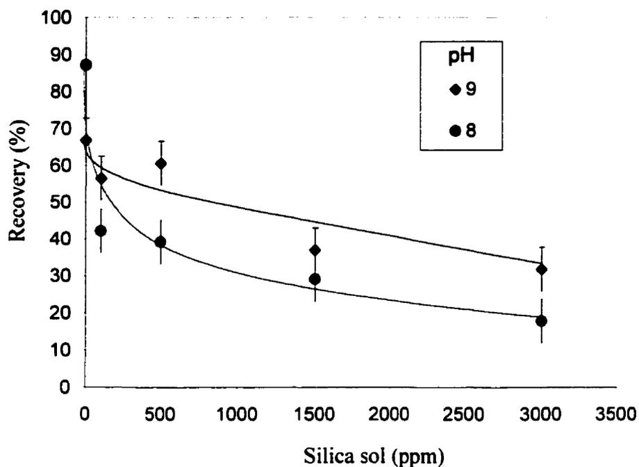
Fig. 4.1 Chalcopyrite recovery as a function of silica sol addition at pH 8 and 9. Note: Error bar is  $2\sigma$ .
