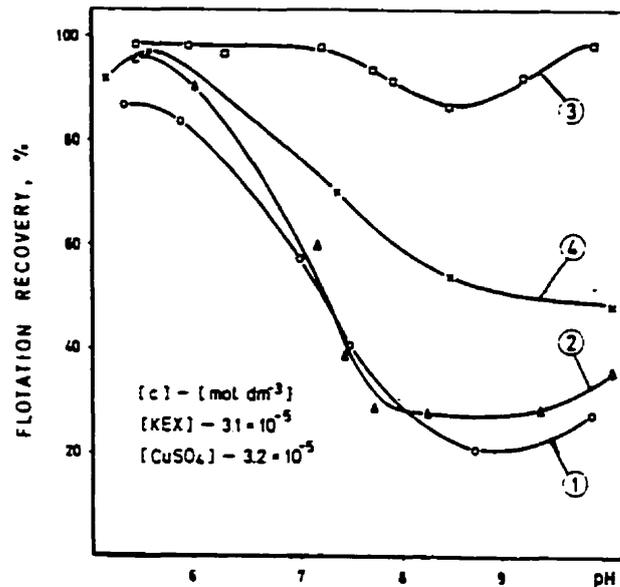
Fig. 2.1 Flotation recovery of sphalerite as a function of pH: 1= No reagents; 2 = CuSO<sub>4</sub>; 3 = CuSO<sub>4</sub> + KEX; 4 = KEX (after: Popov and Vucinic, 1990).
