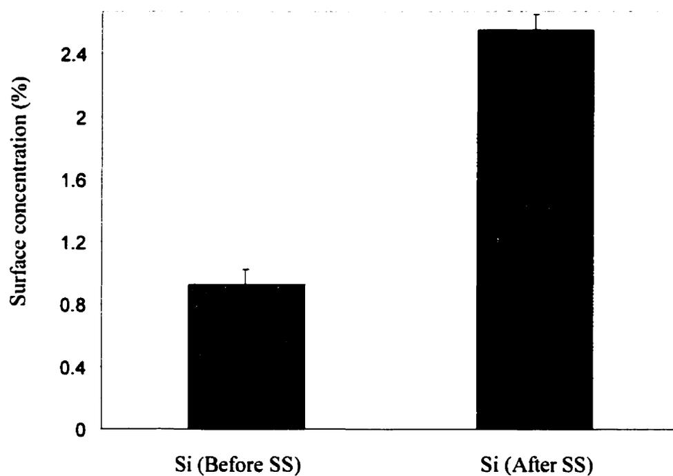
Fig. 4.14 Surface concentration of Si on chalcocite surface before and after silica sol (SS) addition at pH 9. Note: Error bar is  $2\sigma$ .
