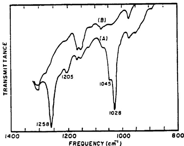
Fig. 2.7 Infrared spectra of pyrite conditioned in the absence of (curve B) and presence of (curve A) of potassium amyl xanthate (after: Fuerstenau et al., 1968).
