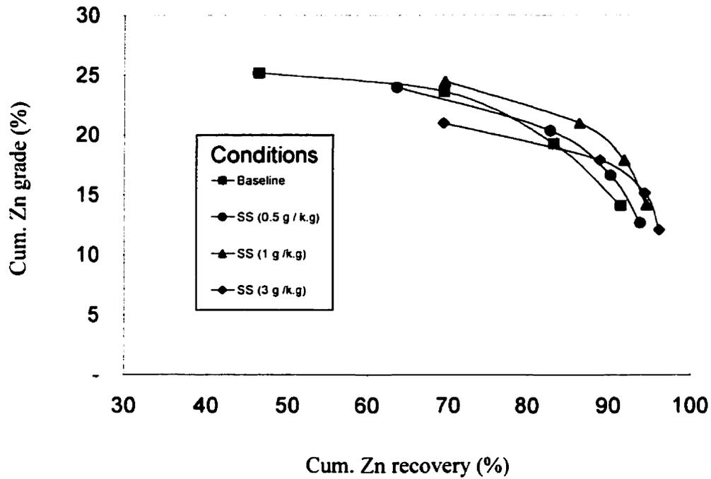
Fig. 4.26 Cumulative Zn grade vs recovery for various concentration of silica sol.
