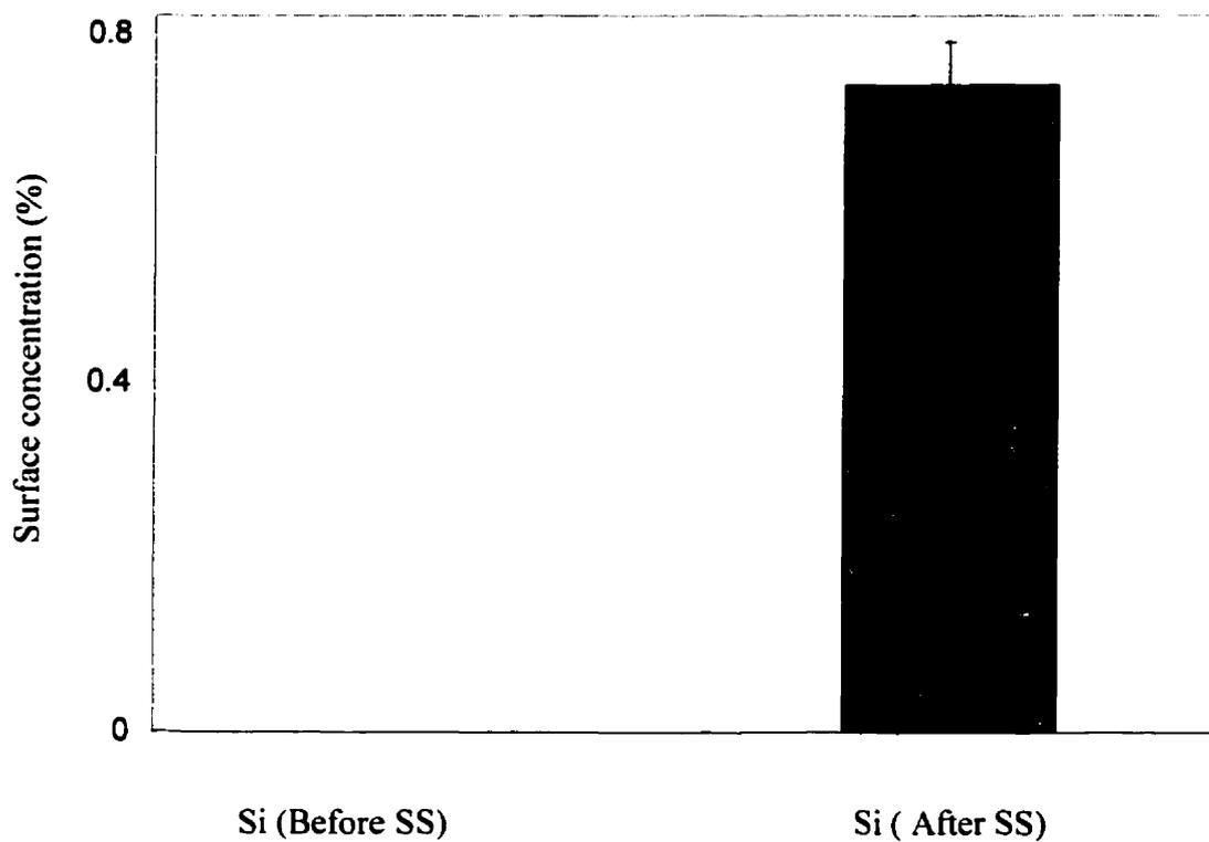
Fig. 4.11 Surface concentration of Si on non activated pyrite surface before and after silica sol (SS) addition at pH 9. Note: Error bar is  $2\sigma$ .
