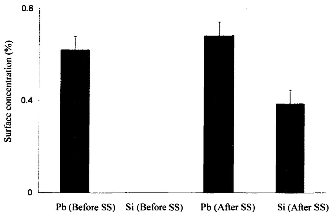
Fig. 4.13 Surface concentration of Pb and Si on Pb activated pyrite surface before and after silica sol (SS) addition at pH 9. Note: Error bar is  $2\sigma$ .
