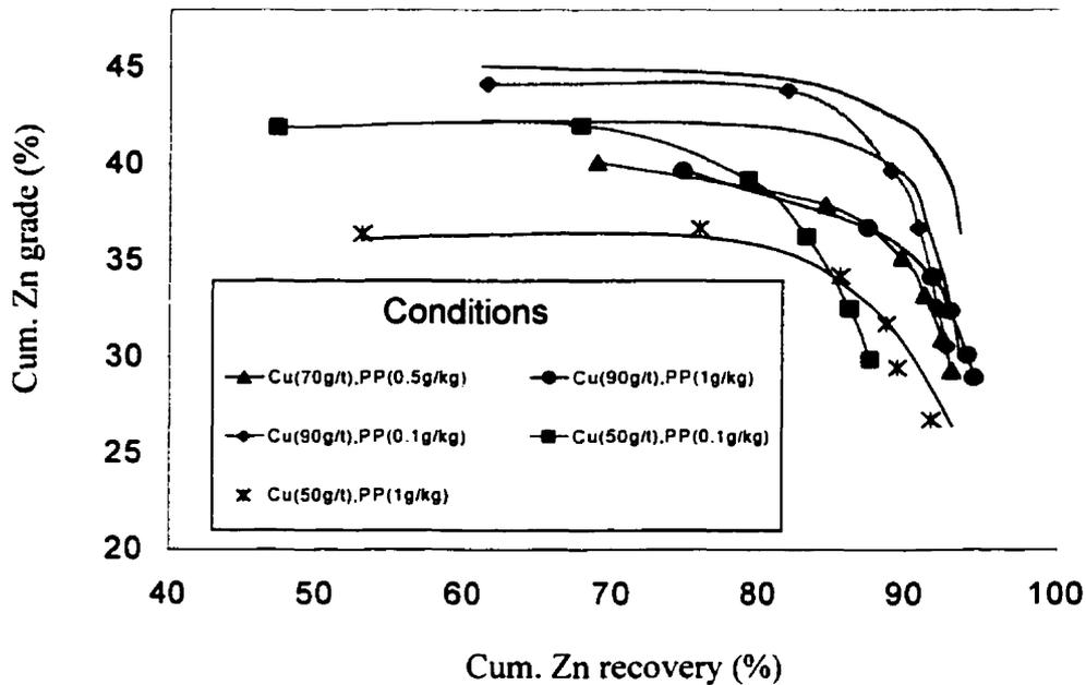
Fig. 4.32 Cumulative Zn grade vs recovery for various combinations of  $\text{CuSO}_4$  and polyphosphate: PP added after  $\text{CuSO}_4$ .
