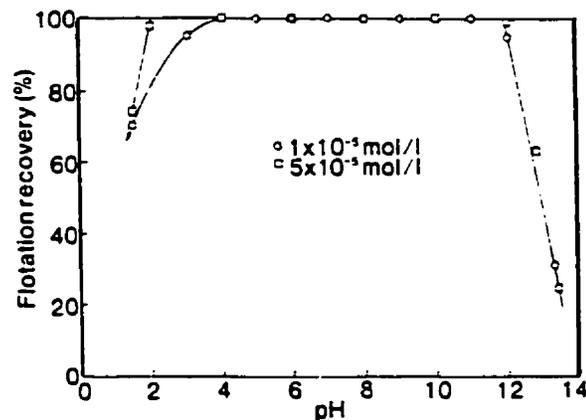
Fig. 2.8 Flotation recovery of chalcopyrite as a function of pH and ethyl xanthate concentration (after: Fuerstenau and Rowse, 1978).
