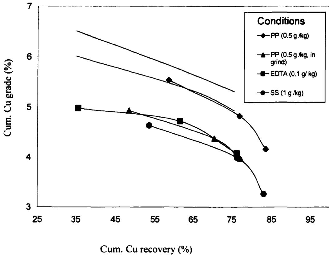
Fig. 4.16 Cumulative Cu recovery vs grade for various conditions: Les Mines Selbaie without NaCN.
