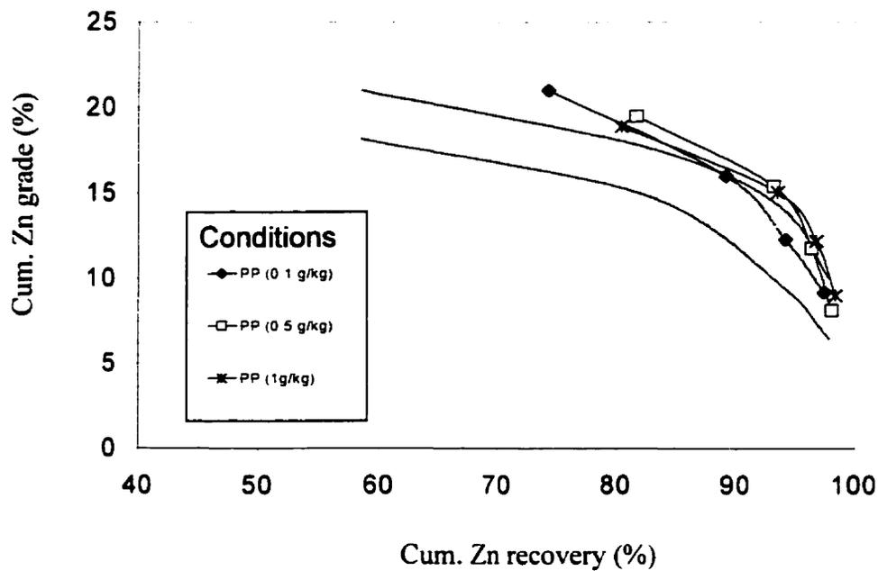
Fig. 4.30 Cumulative Zn grade vs recovery for various concentrations of polyphosphate with recomputed baseline 95 % CI band.
