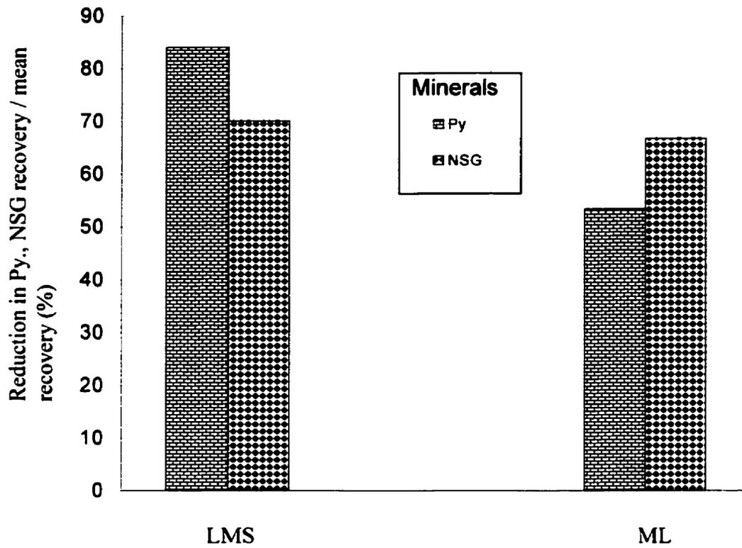
Fig. 5.5 Reduction in pyrite and non sulphide gangue recovery after polyphosphate (0.5 g/kg) addition relative to mean baseline recovery for Les Mines Selbaie (LMS) at 60 % cum. Zn recovery and Mine Louvicourt (ML) at 80 % cum. Zn recovery.
