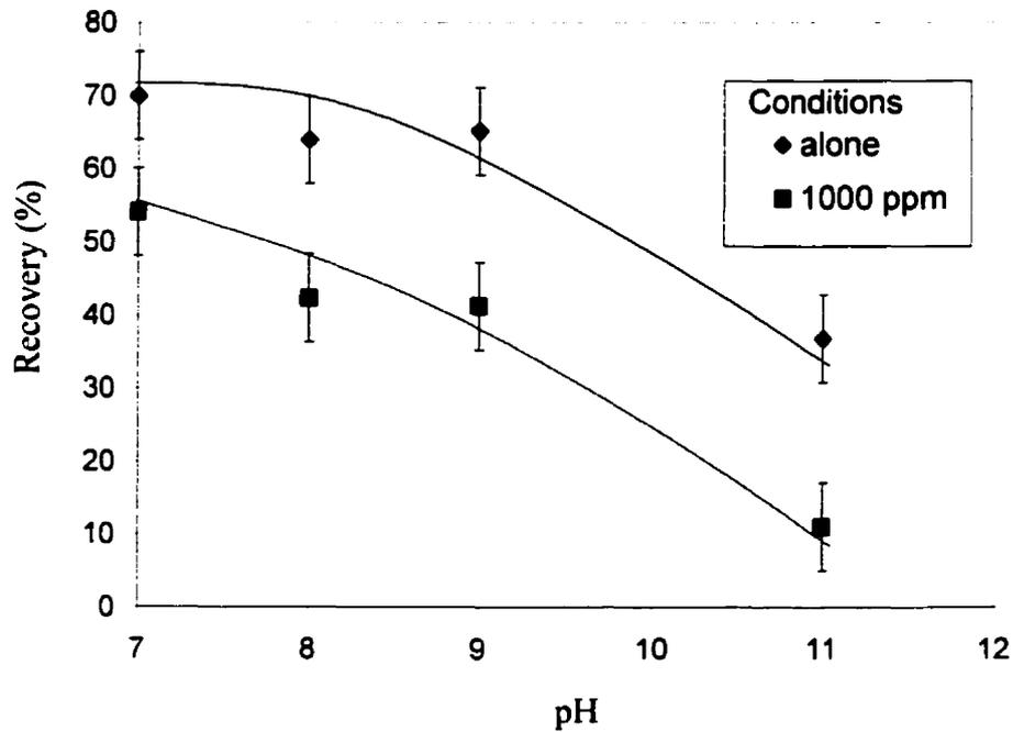
Fig. 4.7 Chalcocite recovery as a function of pH at 1000 ppm of silica sol.
