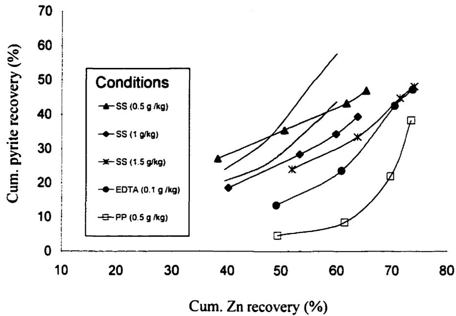
Fig. 4.20 Cumulative pyrite recovery vs Zn recovery for various conditions with NaCN in Cu stage). Note: Pyrite grade was computed from the metal assays allowing for Fe in chalcopyrite and 2 % Fe in sphalerite.
