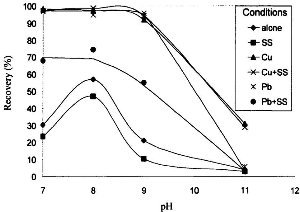
Fig. 4.4 Sphalerite recovery as a function of pH for various conditions. Note:
