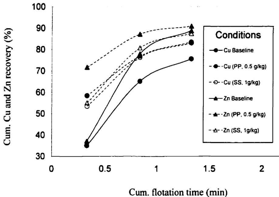
Fig. 4.17 Rate of flotation: Cumulative Cu and Zn recovery vs time with and without polyphosphate and silica sol.
