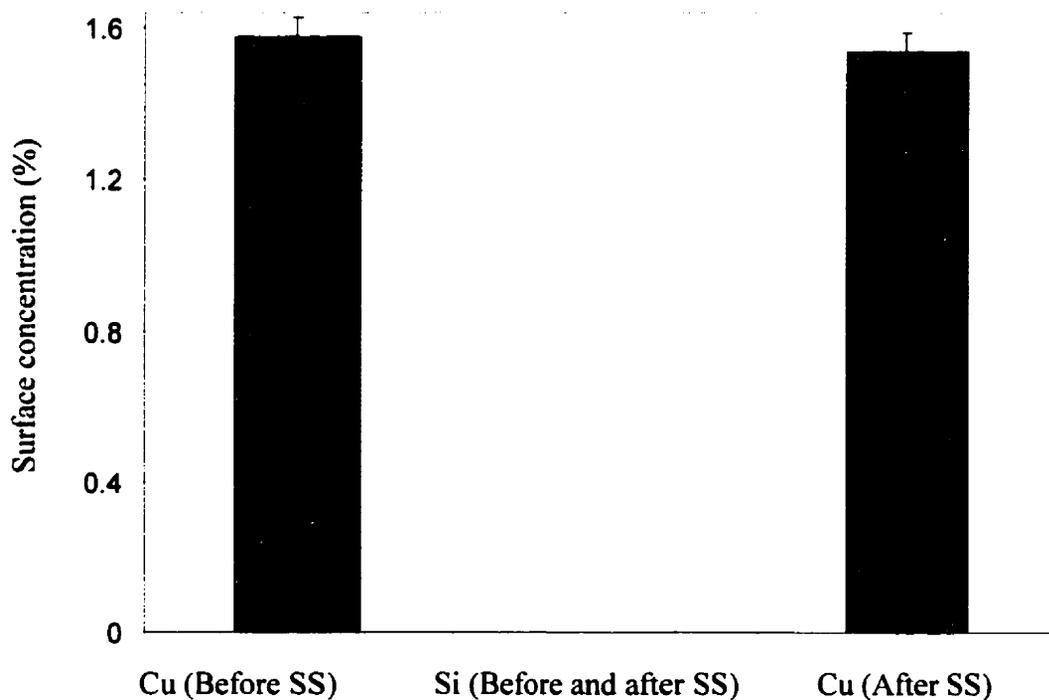
Fig. 4.9 Surface concentration of Cu on Cu activated sphalerite surface before and after silica sol (SS) addition at pH 9. Note: Error bar is  $2\sigma$ .
