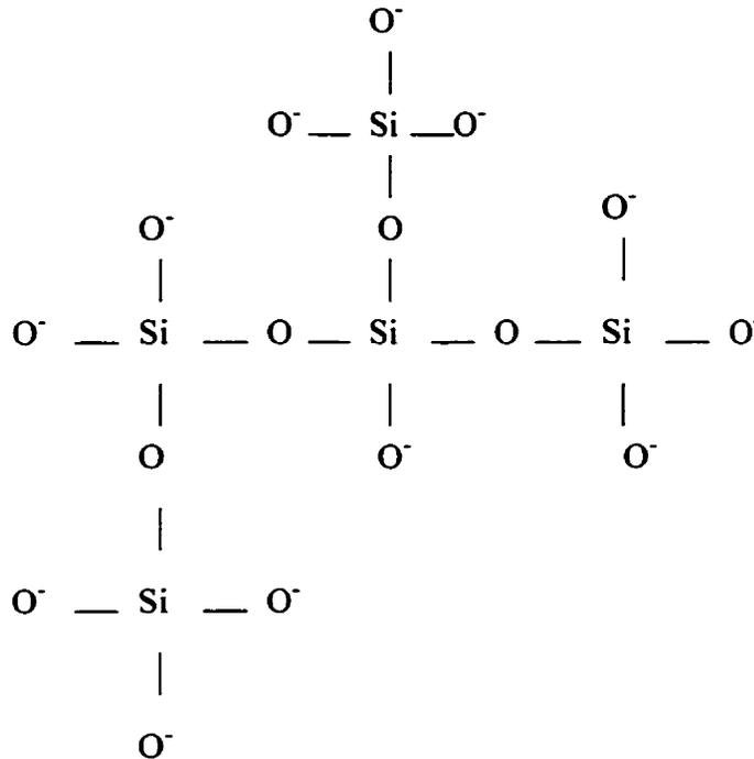
Fig. 1.1 Structure of silica sol
