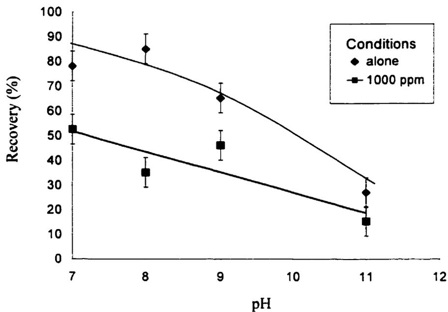
Fig. 4.2 Chalcopyrite recovery as a function of pH with and without 1000 ppm of silica sol. Note: Error bar is  $2\sigma$ .
