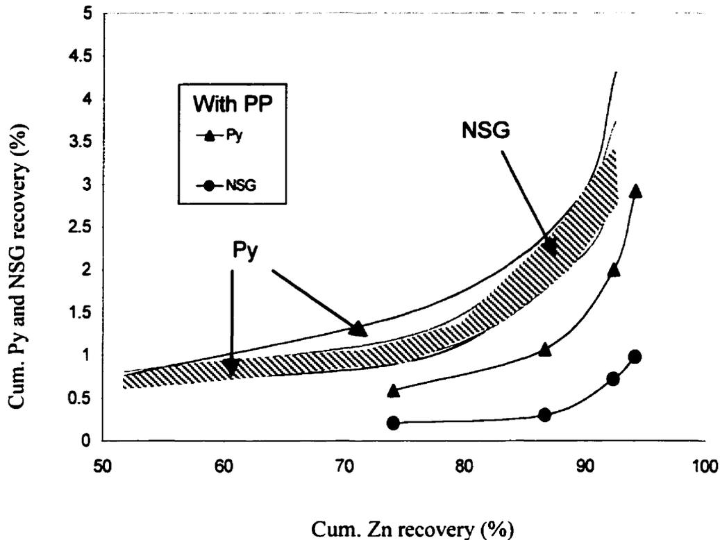
Fig. 5.4 Cumulative pyrite and non sulphide gangue recovery vs Zn recovery for Mine Louvicourt (baseline - shaded area, and with 0.5 g /kg PP - symbols).
