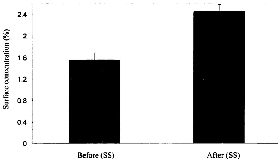
Fig. 4.8 Surface concentration of Si on chalcopyrite surface before and after silica sol (SS) addition at pH 8. Note: Error bar is  $2\sigma$ .
