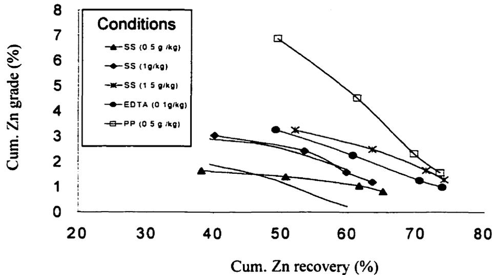
Fig. 4.19 Cumulative Zn grade vs recovery for various conditions (with NaCN in Cu stage).
