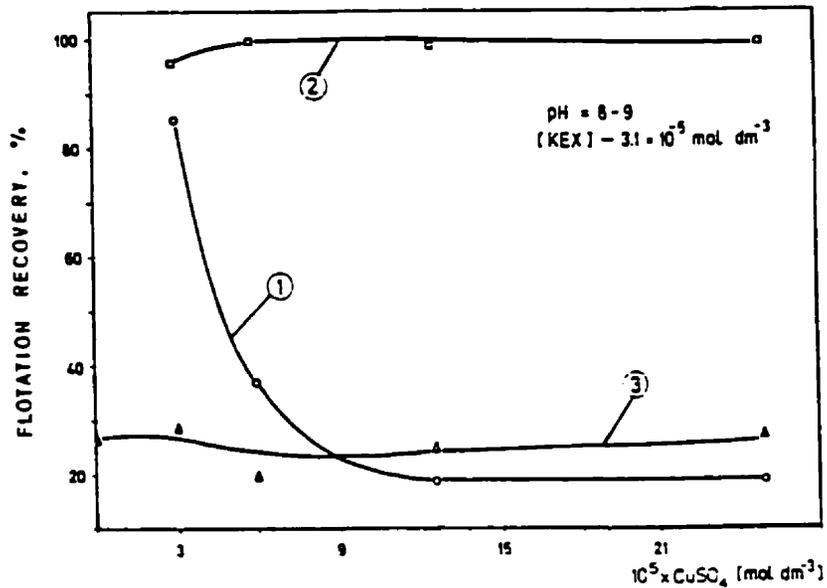
Fig. 2.2 Flotation recovery of sphalerite as a function of  $\text{CuSO}_4$ : 1 =  $\text{CuSO}_4$  (without decantation) + KEX; 2 =  $\text{CuSO}_4$  (decantation) + KEX; 3 =  $\text{CuSO}_4$  (after: Popov and Vucinic, 1990).
