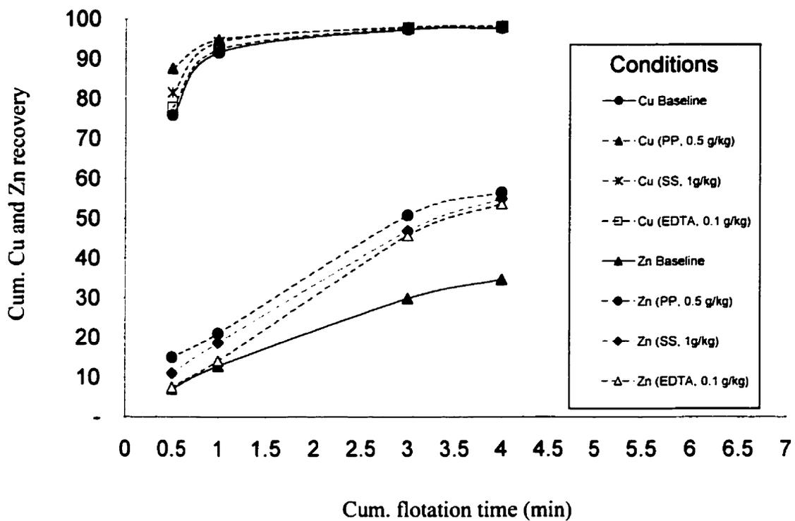
Fig. 4.22 Rate of flotation: Cumulative Cu and Zn recovery vs time with and without polyphosphate, silica sol and EDTA.
