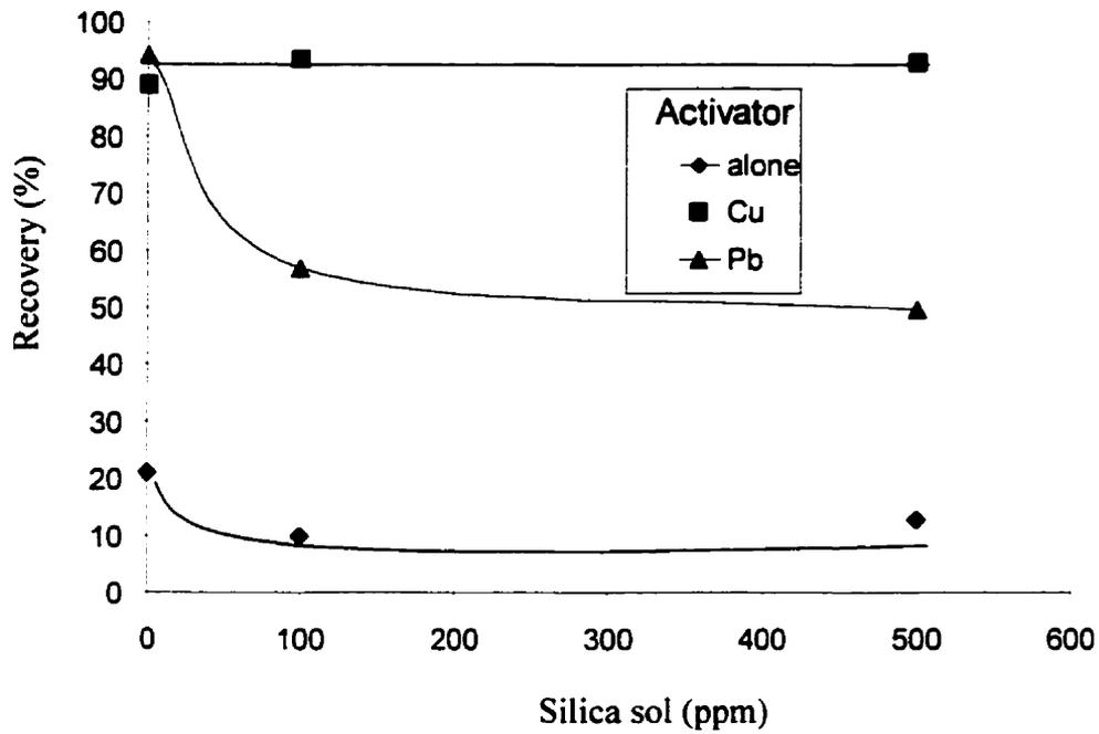
Fig. 4.3 Sphalerite recovery as function of silica sol addition at pH 9.
