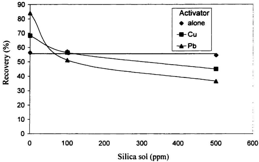
Fig. 4.5 Pyrite recovery as a function of silica sol addition at pH 9.
