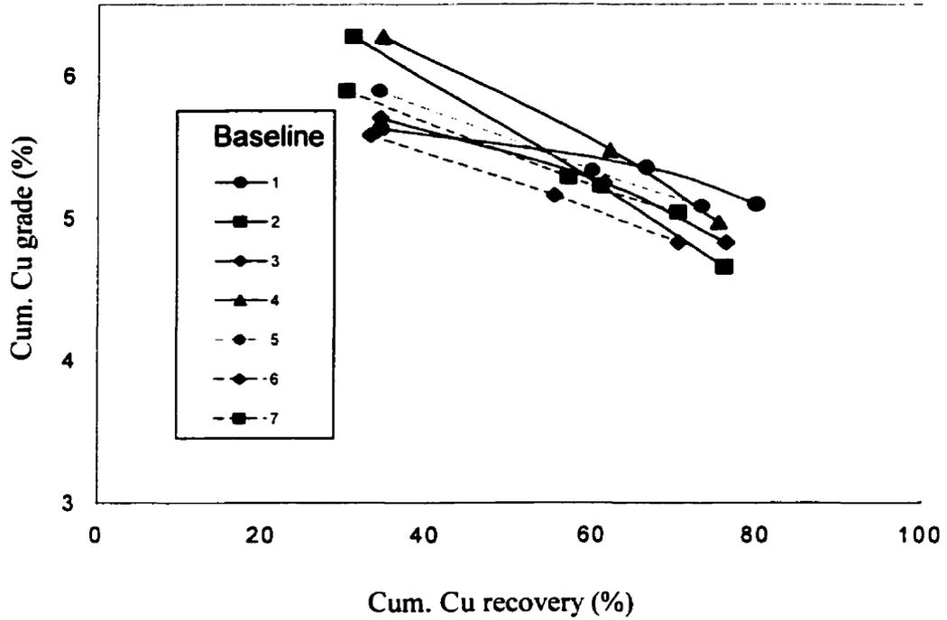
Fig. 4.15a Repeatability: Baseline cumulative Cu grade vs recovery test results - Les Mines selbaie with NaCN added in grinding.
