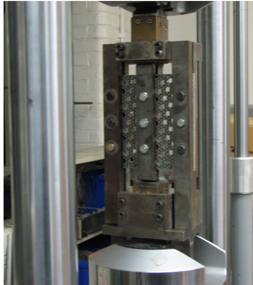
Fig (6.3) Shear specimen mounted into the three rail shear fixture and installed into the test machine
