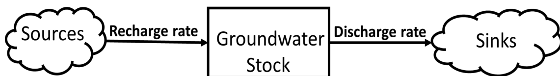
Figure 5.1 An example stock-flow diagram of the groundwater system. The clouds represent the sources and sinks, which are surface water in this system. The rectangle is the stock of groundwater and the solid arrows represent inflow and outflow (to the groundwater stock), thus
