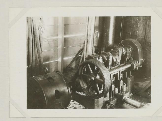
Fig. 16. Stationary electric sprayer for main field experiments, capacity 32 gallons per minute at 650 pounds pressure per square inch. This machine operates four spray guns.
