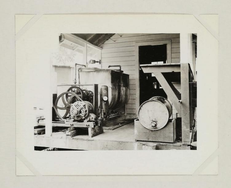
Fig. 15. Stationary electric sprayer for preliminary field experiments, capacity 16 gallons per minute at 450 pounds pressure per square inch. This machine operates two spray guns.
