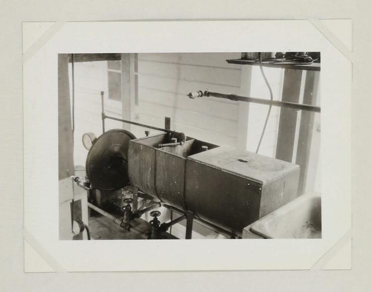
Fig. 14. Laboratory sprayer, showing divided spray tank and valves. Capacity 2-3 gallons per minute at 350 pounds pressure per square inch.
