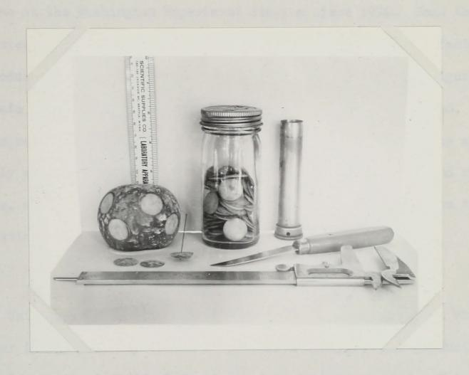
Fig. 1. Equipment for preparation and storage of sample discs for deposit determinations. Left background, an apple with discs removed.
