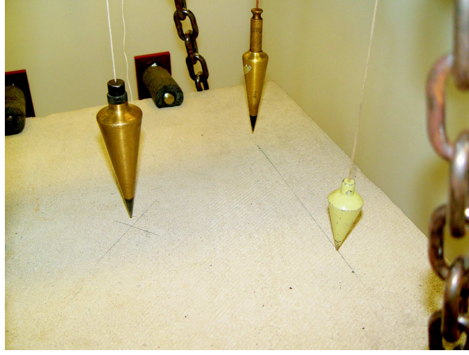
Figure 18: Method for centrally locating the sample with respect to the coordinate system of the reaction frame.
