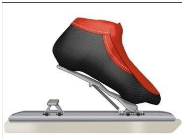
Figure 7: Representation of the Klapskate allowing a greater plantar flexion (adapted from www.quebec-amerique.com ).
