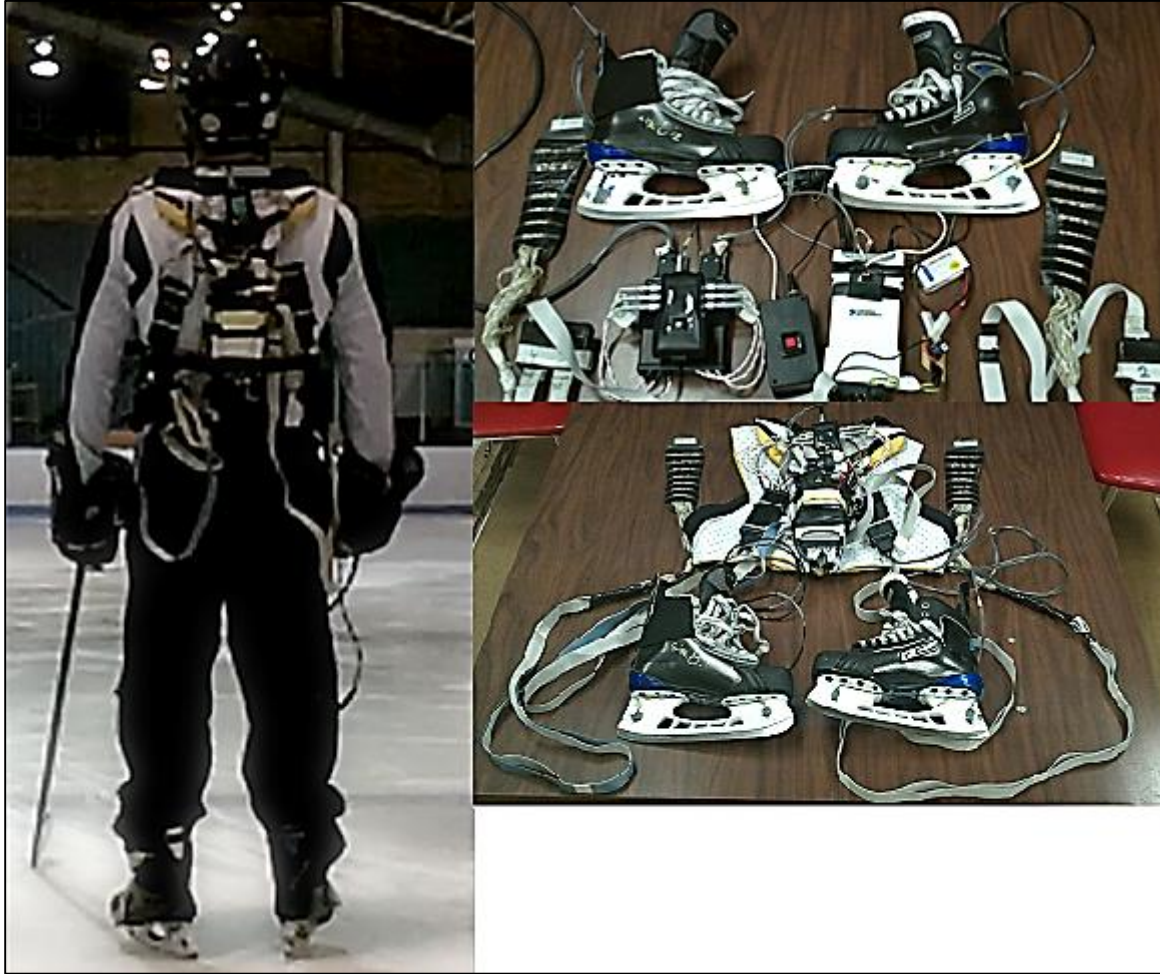
Figure 8: Representation of both skate models instrumented with both wireless systems (top right) with the shoulder pads configuration (bottom right) and the shoulder pads configuration during testing (left).
