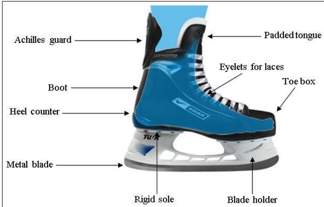
Figure 2: Structural components of a regular hockey skate (adapted from Pearsall and Turcotte, 2007).
