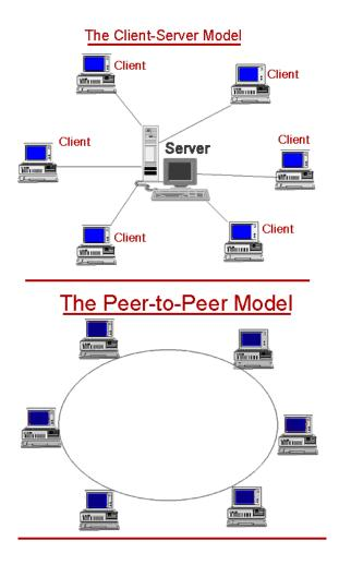
The lines in the diagram represent the flow of data; for BitTorrent, that would be the movie or television or music files being downloaded. Whereas in the client-server model it is easy to see how shutting down the server would stop the flow of information, this would be quite difficult in a P2P model. This becomes even clearer with another, perhaps more accurate, diagram of a P2P model:<sup>29</sup>
