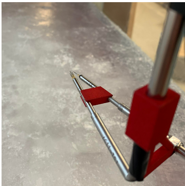
Figure 3.7: Simultaneous operation of an X-wire (left) and cold-wire (right). The X-wire is aligned with the mean flow, while the cold-wire is angled by 12^\circ relative to the mean flow since it is insensitive to changes in velocity.
