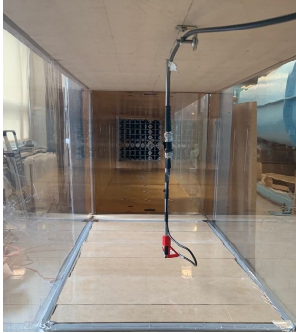
Figure 3.12: Empty tunnel setup for baseline measurements.
