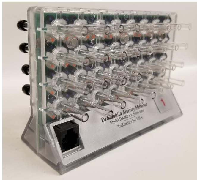
Figure 1.9. Drosophila Activity Monitor. Each glass tubes would contain one adult fly, food at the far end and a cotton plug.
