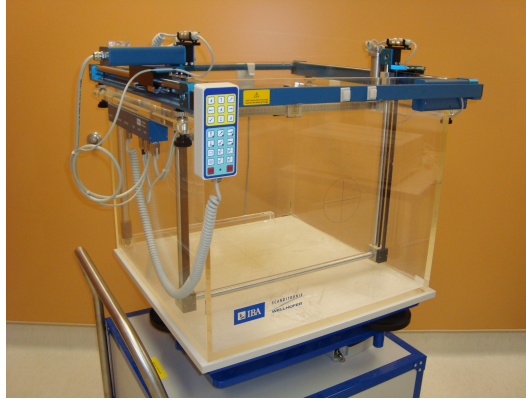
FIGURE 5–1 – Photo of an IBA Blue Phantom water tank with lift table [2].
