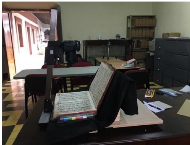
Figure 3-2: Book cradle and camera setup of the DIY book scanner.
