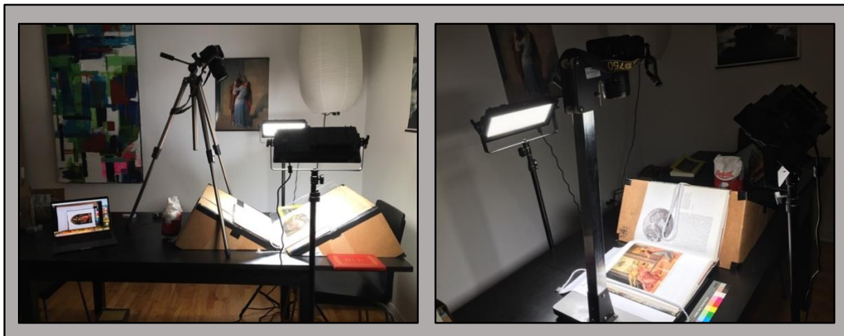
Figure 3-4: At home tests with a cardboard box cut diagonally in half to obtain two big wedges for the book to rest open. I used the two wedges for testing the facing-up V-shaped configuration (left) with the camera placed on the borrowed tripod. I took pictures with and without a platen. I only used one wedge to test the open-at-one-side configuration with the borrowed copystand, with a flexible snake weight to keep the pages resting in the wedge from falling on top of the photographed page.
