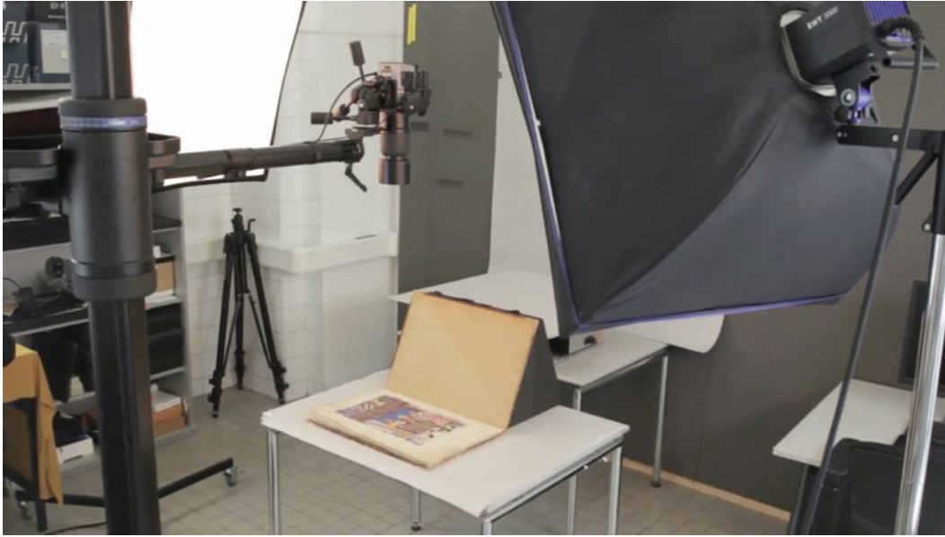
Figure 2-9: Opening the book at one side for digitization of one page at a time. The camera is placed on top of the page to be digitized using a sturdy tripod and a horizontal arm. Lights are positioned at each side of the page for even distribution and at an angle to avoid reflections. Image from https://www.bsb-muenchen.de/einblicke/vom-buch-zum-byte-digitalisierung-an-der-bayerischen-staatsbibliothek/ .
