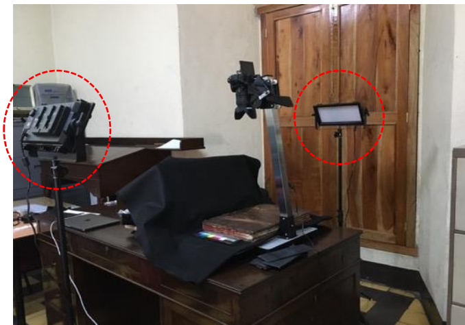
Figure 3-3: DIY book scanner light setup, one on each side for even distribution of the light over the page.
