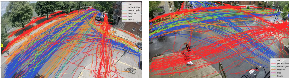
Figure 3-3 Trajectories tracked by computer vision of the commercial software corresponding to the intersections in Figure 3-2
