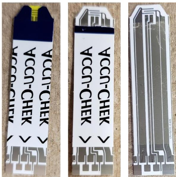
**Figure 5.1 Components of Accu-chek aviva test strips:** Photograph of the unmodified test strip before (left) and after (right) peeling off the protecting cover and removing the enzyme (middle)
