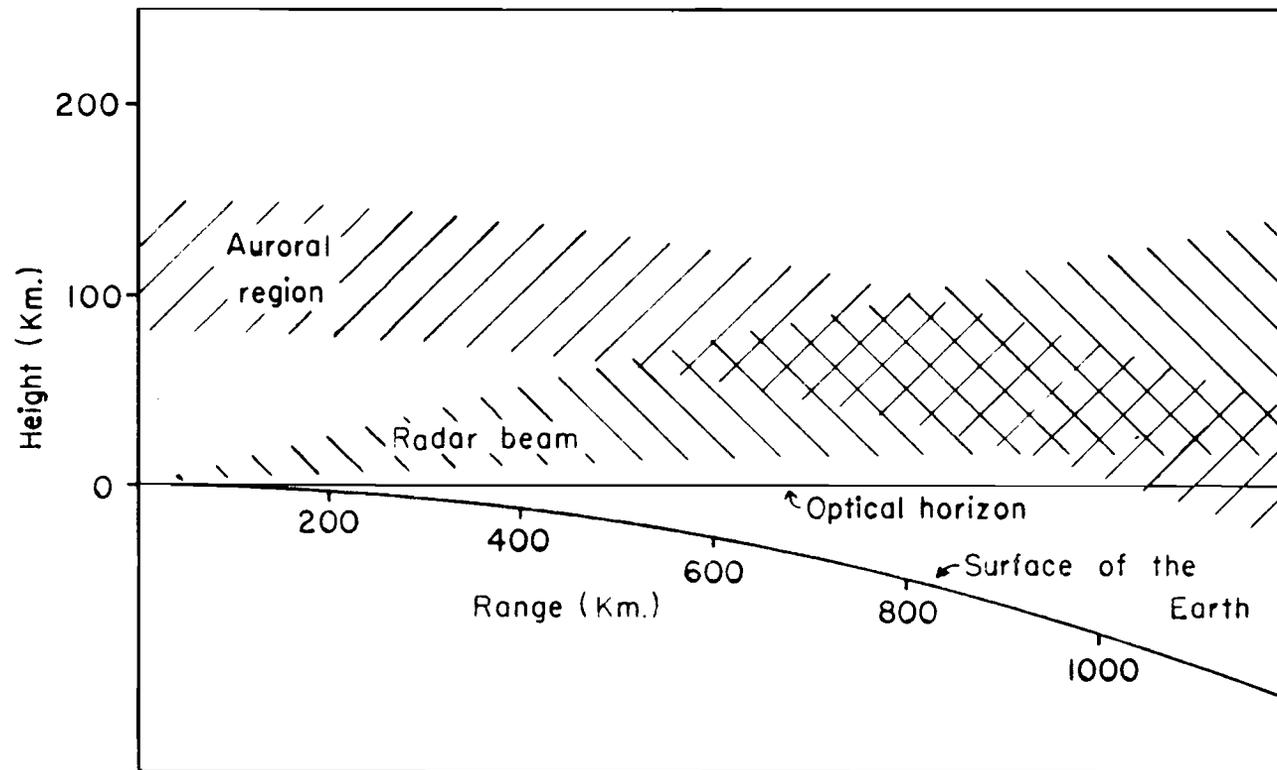
Figure 3.01 - Schematic diagram showing vertical section through the auroral region and the radar beam.
