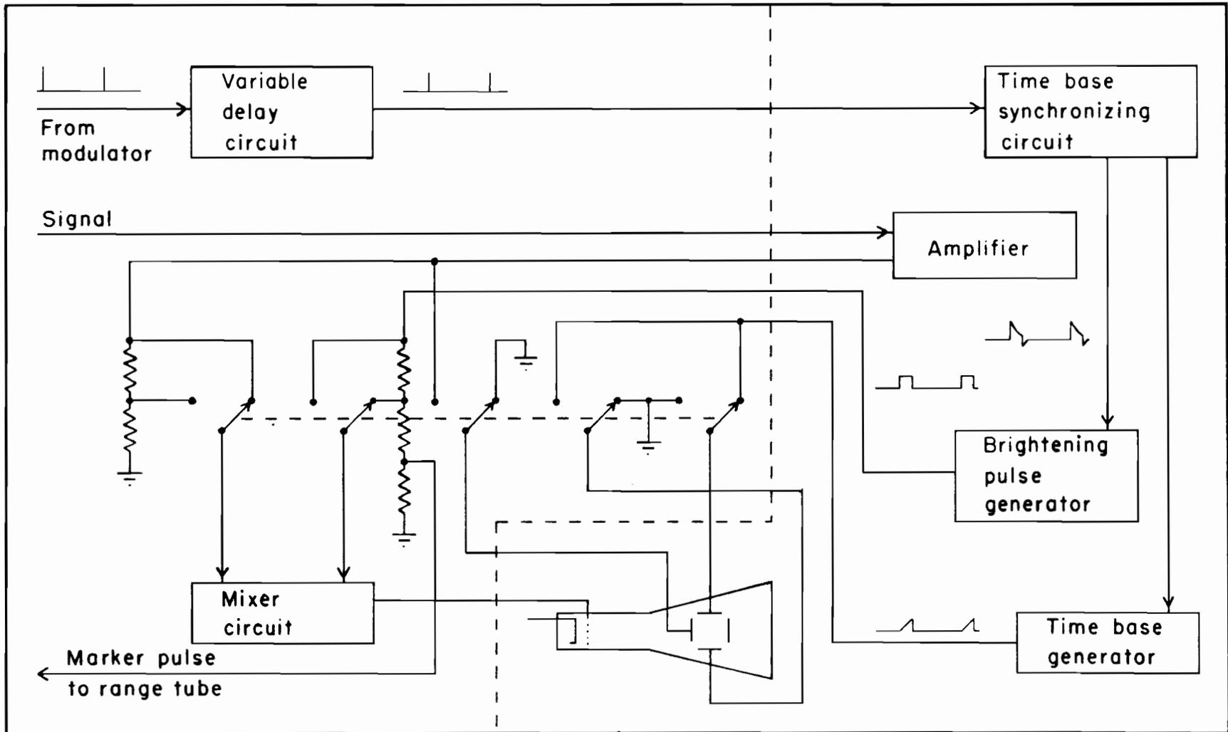
Figure A2.04 - Schematic diagram of the equipment used for continuous recording of auroral echoes.
