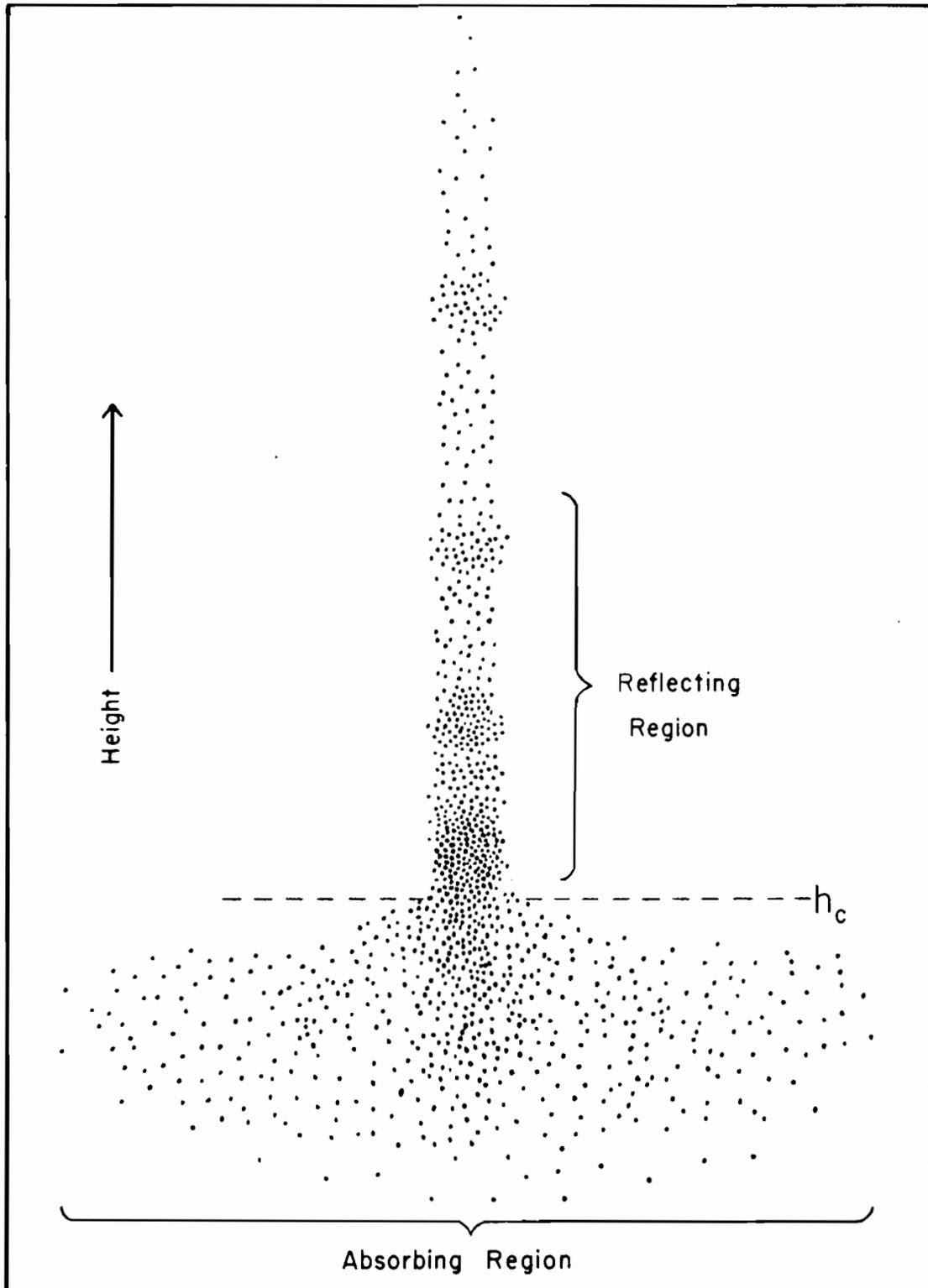
Figure 5.05 - A schematic diagram of the suggested electron distribution in a reflecting centre.
