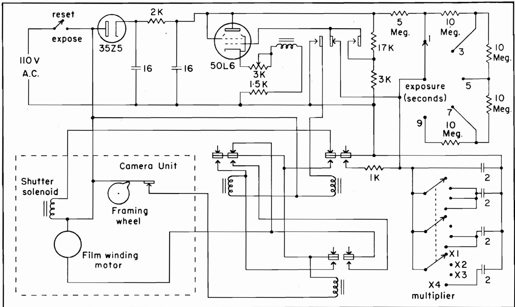
Figure A2.01 - Schematic diagram of the remotely controlled auroral camera.
