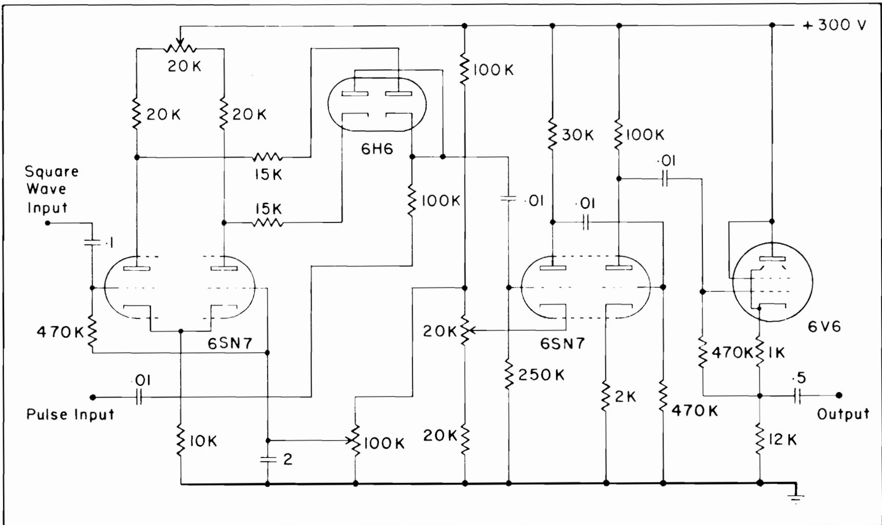
Figure A2.03 - Circuit diagram of the pulse selector.
