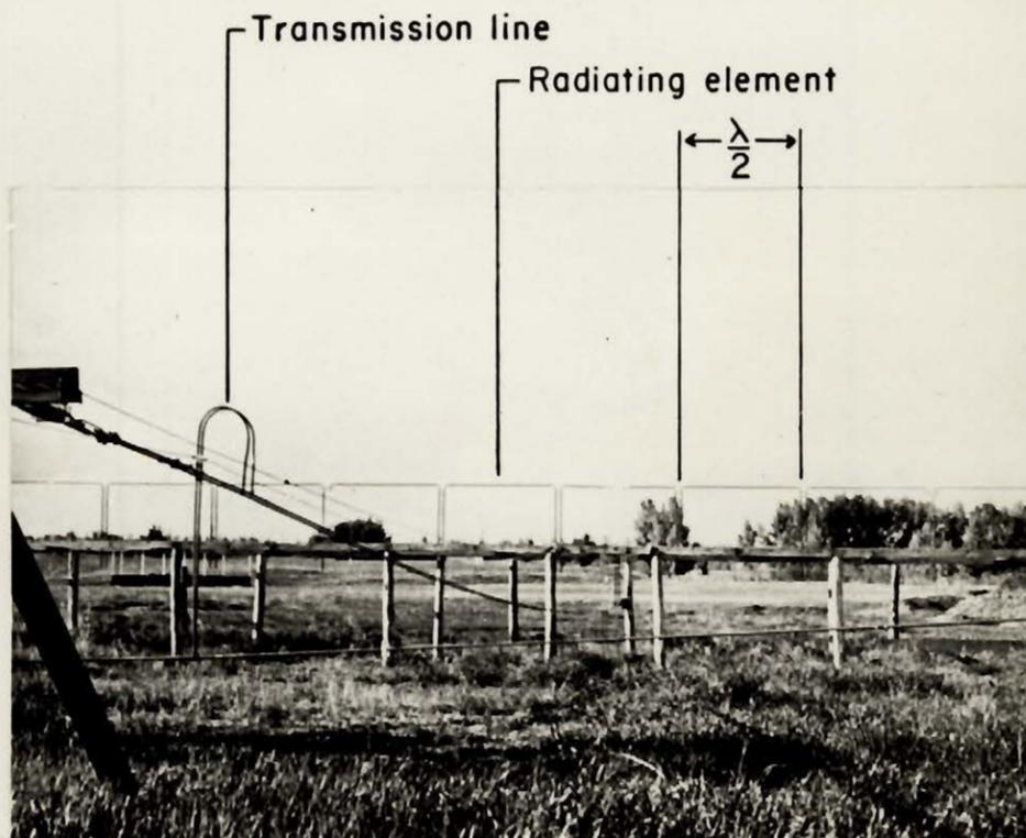
Figure 5.01 - The aerial array used for high-angle observations.
