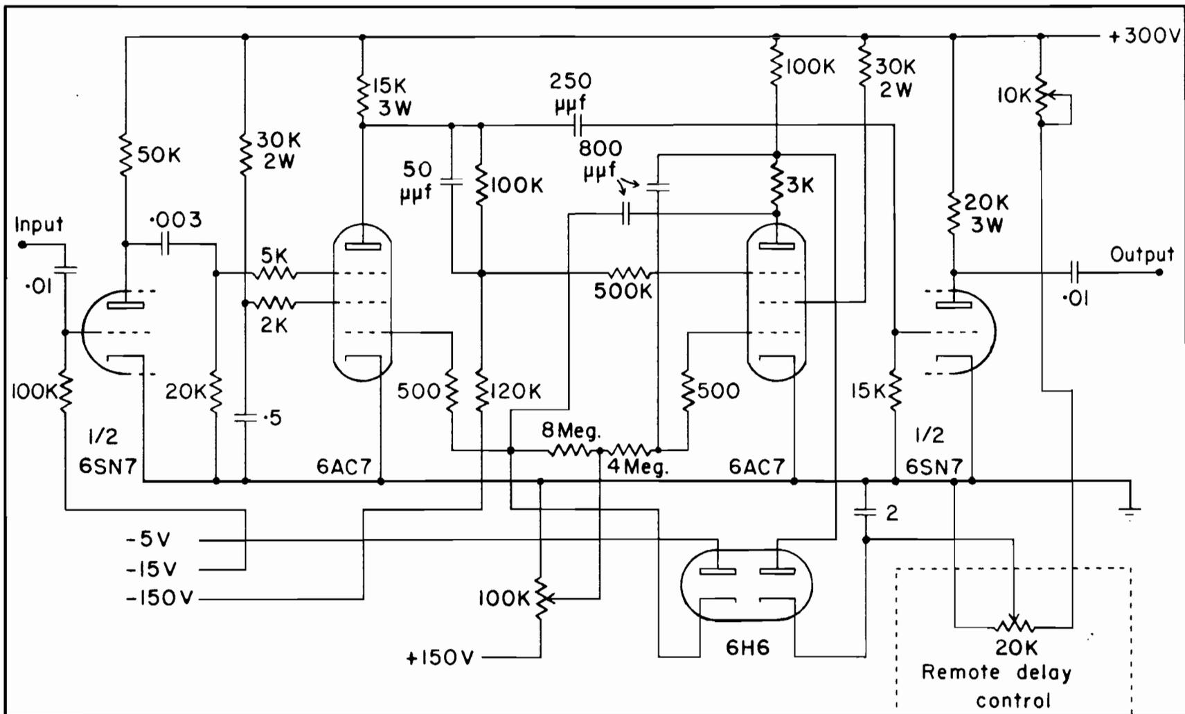
Figure A2.05 - Circuit diagram of the variable delay unit.
