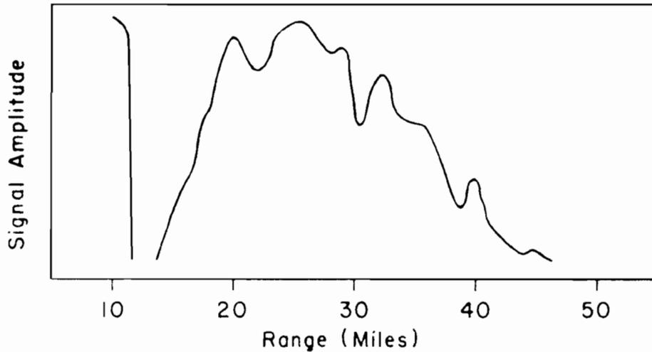
Figure 4.02 (b) - Amplitude of echo from aircraft at an altitude of 10,300 feet.
