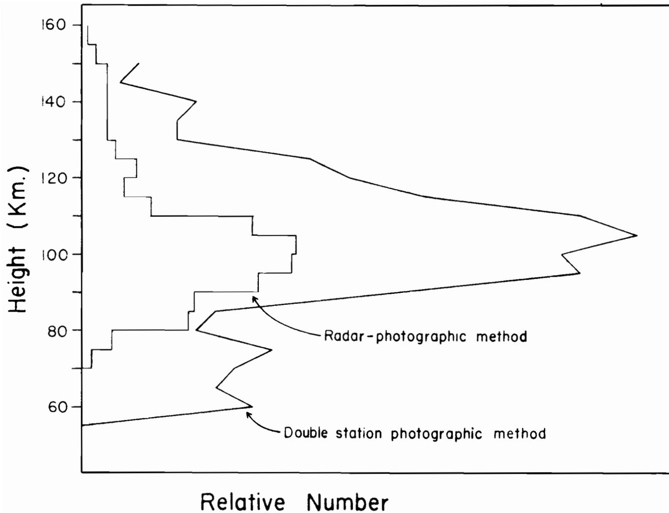
Figure 3.08 - Distribution of frequency of occurrence with height as found by Alty and Wilson (double station photographic method) and as found by the radar-photographic method.
