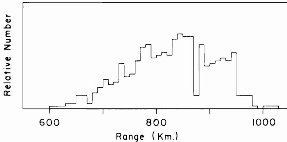
Figure 4.02 (a) - Frequency of occurrence of auroral echoes for azimuth sector  $350^{\circ} - 010^{\circ}$ .
