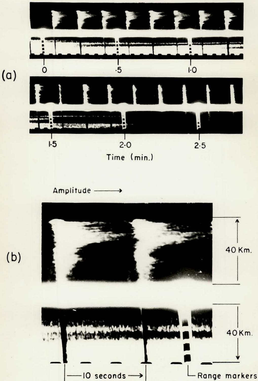
Figure 5.08 - Continuous record showing the variation in amplitude and range of auroral echoes.
