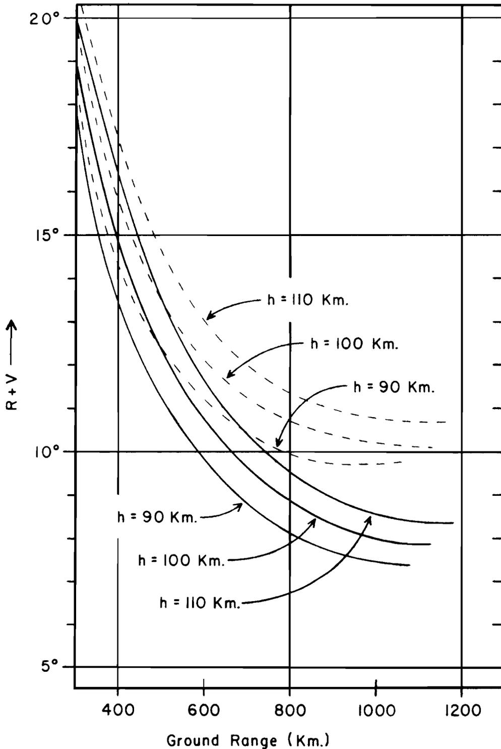
Figure 4.06 - Showing the angle of inclination,  $(R + V)$ , of rays at the reflection level. Solid lines refer to propagation in the standard atmosphere, broken lines to a non-refracting atmosphere.
