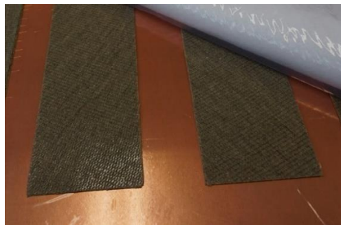
FIGURE 7: FLAXPREG UD 180 PREPREG FROM LINEO.
