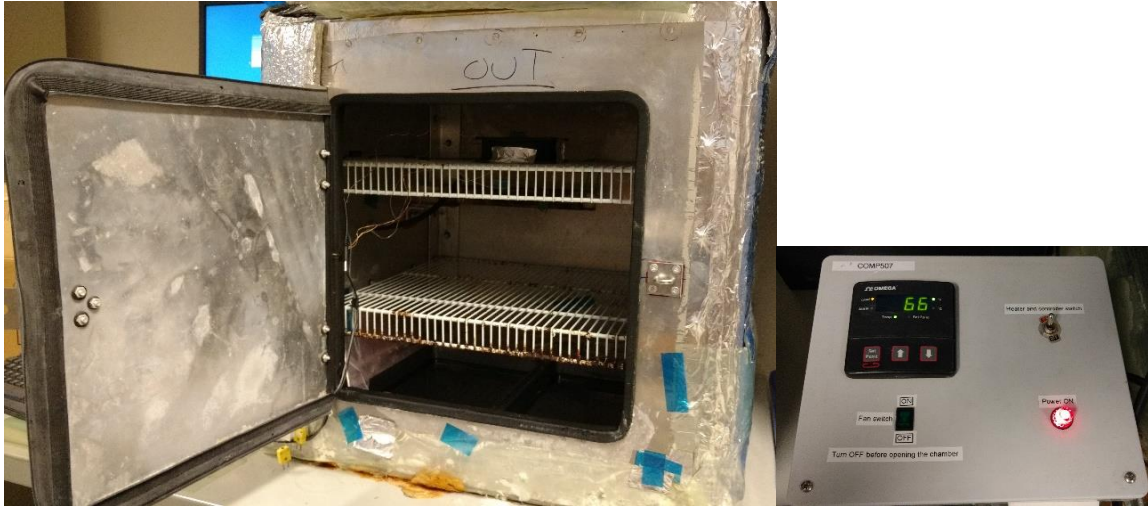
HUMIDIFYING CHAMBER AND CONTROLLER BUILD IN THE LAB.
