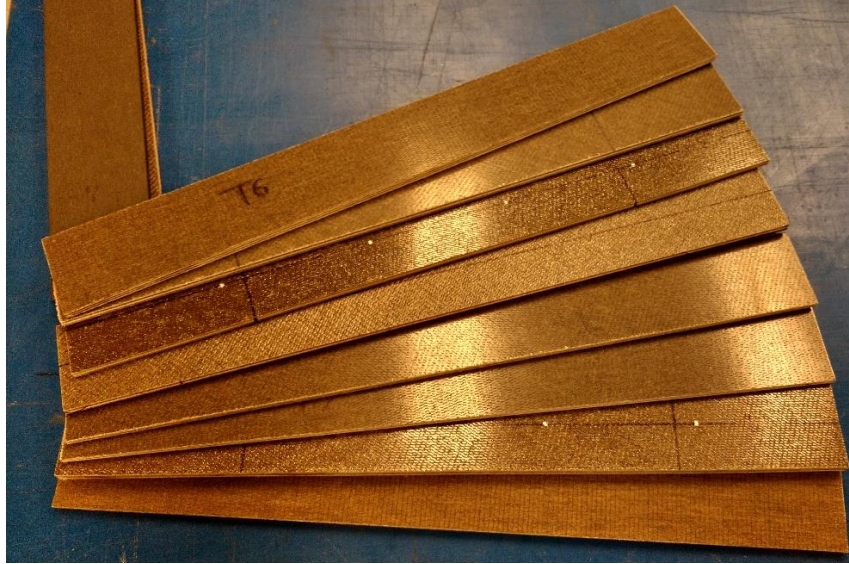
FIGURE 15: FLAX FRETBOARD SAMPLES MANUFACTURED.
