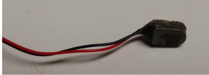
FIGURE 11: PCB PIEZOTRONICS MODEL 352A73 ACCELEROMETER SENSOR.
