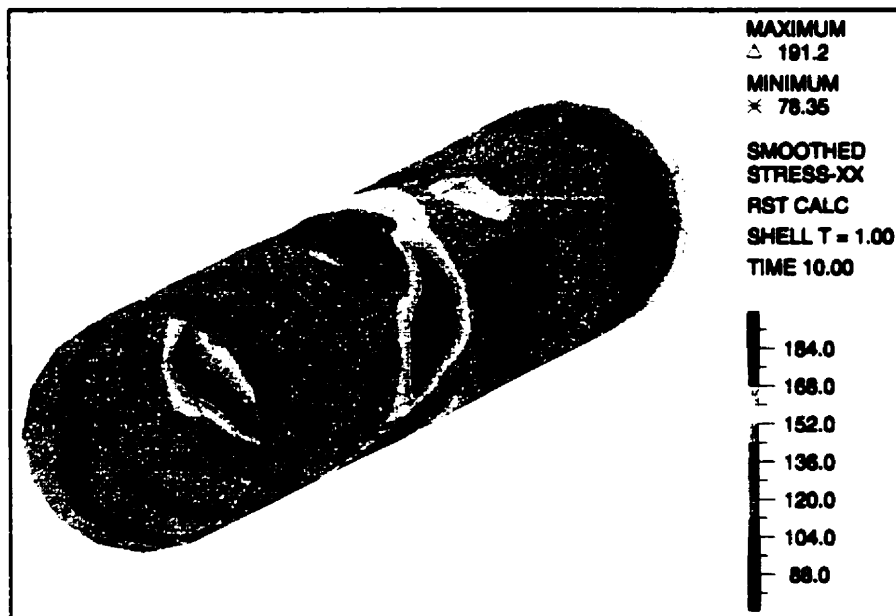
Figure 5.77 Stress distribution in central tube
