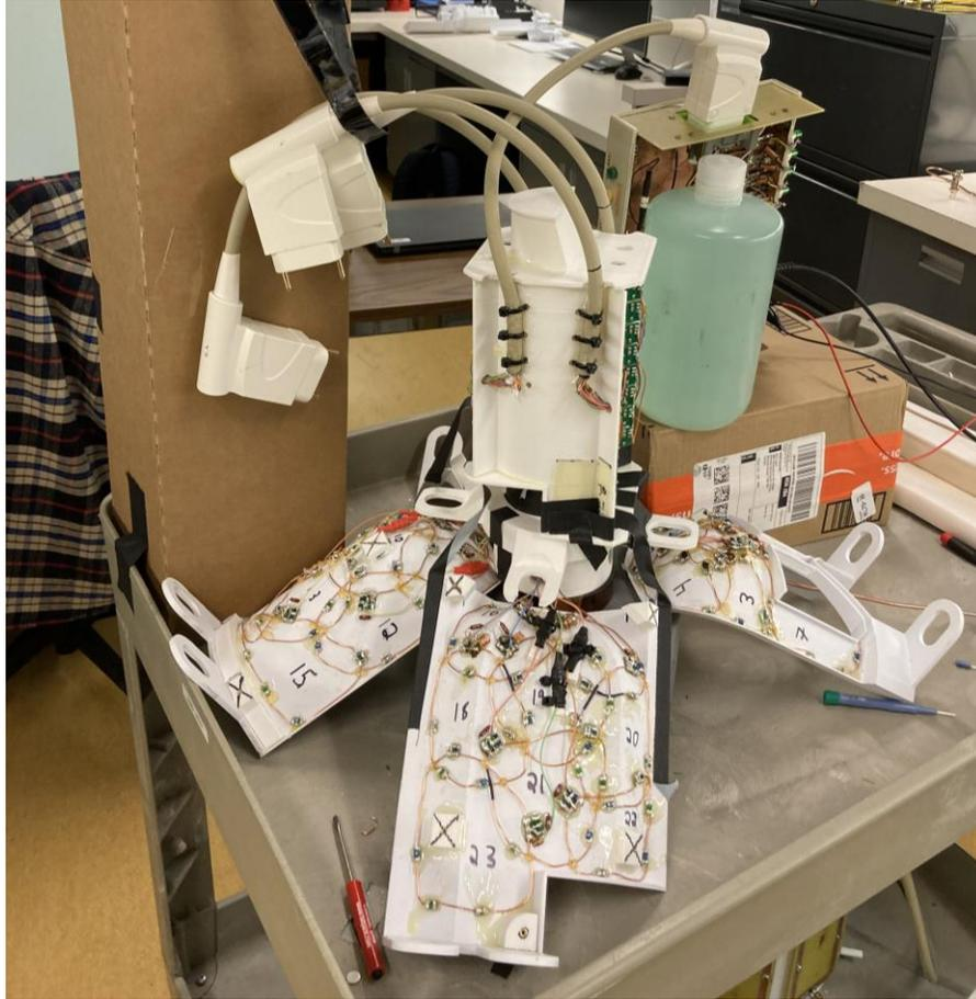
*Figure 21: Testing setup used to optimize performance of individual Rx array elements. Since cabling from each component of the Rx former was fed to a single mechanical structure housing the preamplifiers at the top of the coil, optimization of elements required some disassembly of the adjustable pieces. Future designs are seeking to improve the stability of electrical and mechanical components of the size adjustable array design.*
