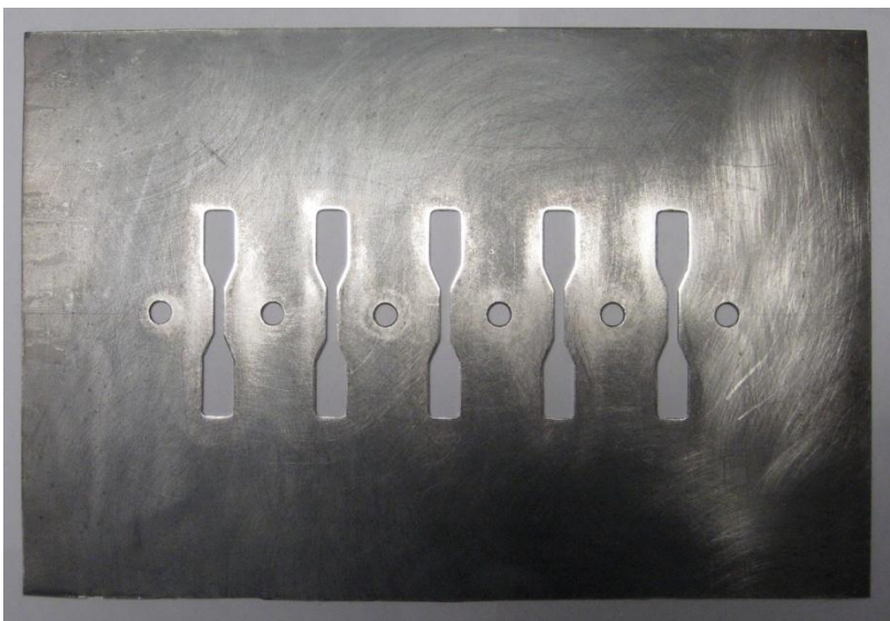
Figure 8 - Mould for preparation of 5 tensile strength test bars
