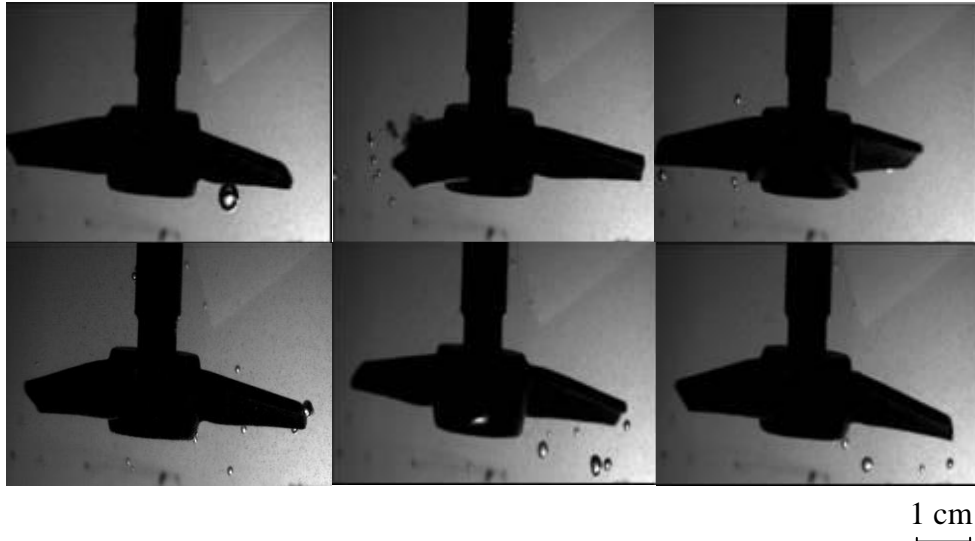
Figure 3.8: Sequence of images recording one-bubble-at-a-time break-up event in the presence of 0.047 mmol/L (20 ppm) F150
