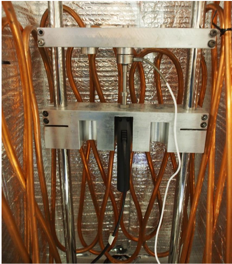
Figure 13 Stress-Strain device, used for thickness measurement
