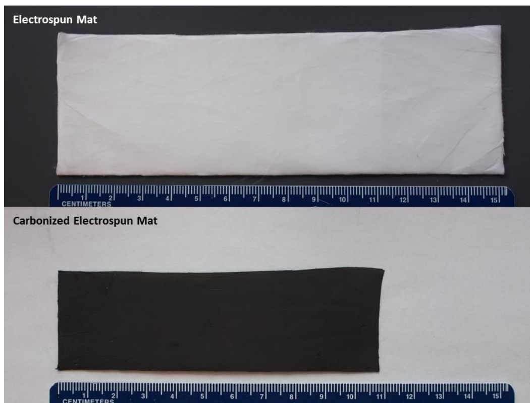
Figure 19 Images of electrospun PAN mat before and after carbonization
