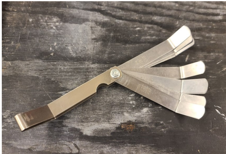
Figure 4.4: Feeler gauge used in the Rock bolting laboratory.
