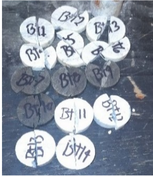
Figure 5.3: Barite BTS tested samples. Note: samples BT7 to BT10 show a different mineral composition.
