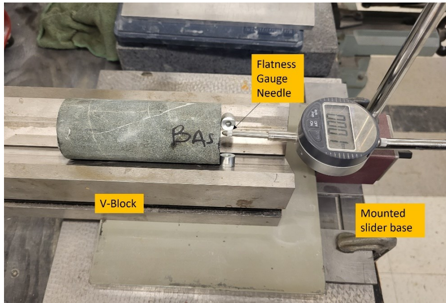
Figure 4.5: V-block apparatus used in the Rock bolting laboratory.
