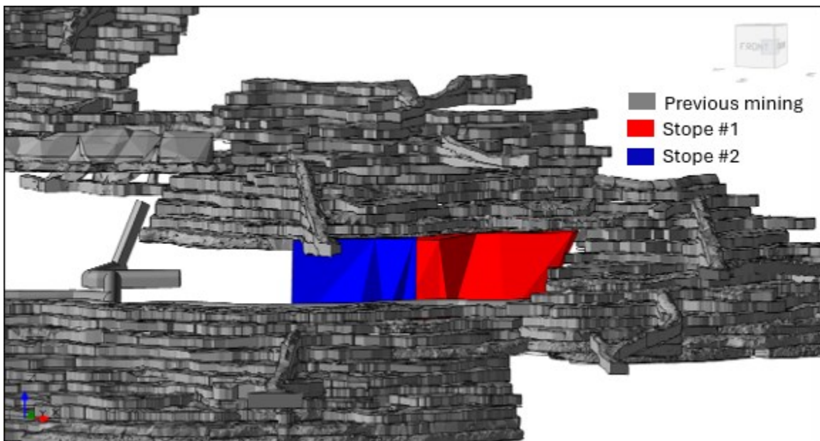
Figure 3.3: Front view of the Stopes located on the sill pillar.
