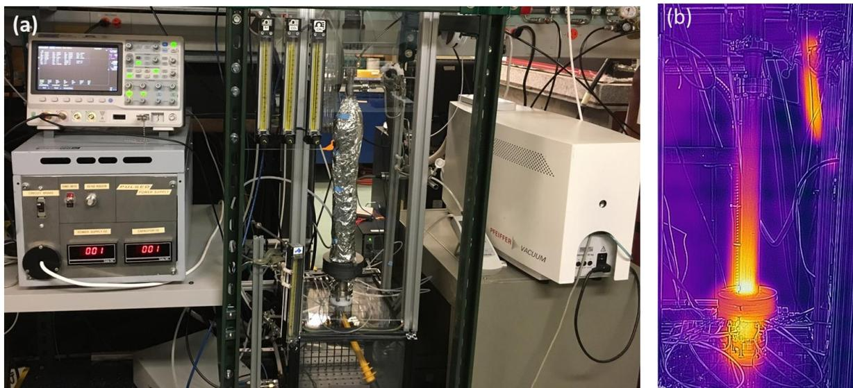
Fig. 3-1 (a) Photograph of the RGA setup. (b) Infrared photograph of the RGA reactor during DRM reaction. Taken with Cat S61 FLIR camera.
