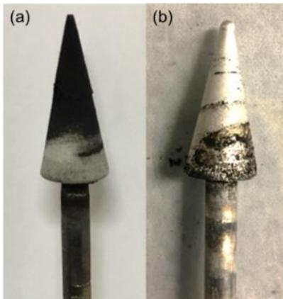
Fig. 6-6 Stainless steel cathode after DRM reaction under (a) plasma-only and (b) plasma-catalytic conditions.
