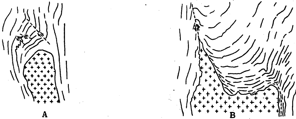
Figure 37. Deformation of schist at the end of two dykes in the Homestake Mine, South Dakota. The schists have been thrust aside and ahead of the advancing magma and have been displaced along small faults. In B the magma subsequently advanced along one of these faults. The dyke in A is about 15 inches wide, that in B about 7 feet wide. A is a plan, B a vertical section(after Noble, 1952).
