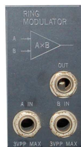
Fig. B.8 Ring modulator interface of the Korg MS-50
