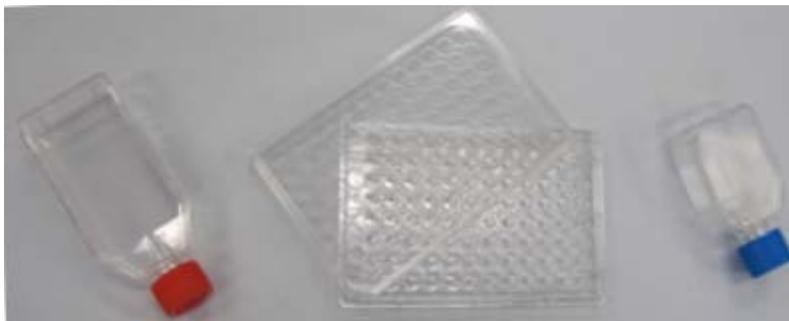
**Fig. 2.1: Cell Culture Vessels: T-25, 96-well Microplate with cover, and T-12.**
