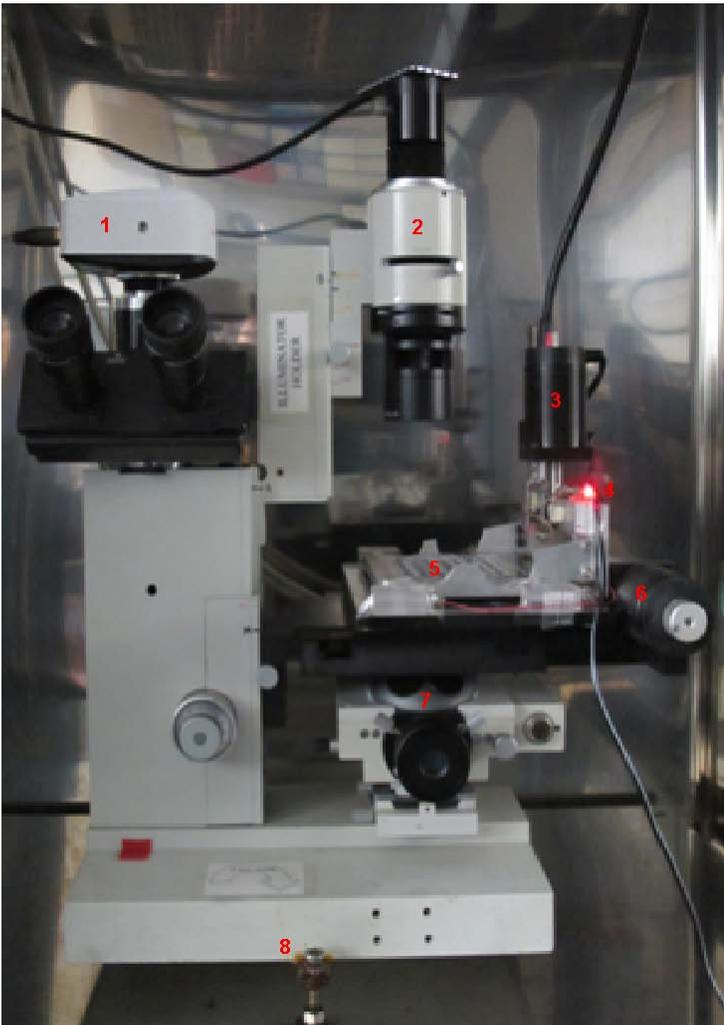
In *manual assays*, T-25s were successively placed at time intervals on the motorized stage (Marzhauser MCL) mounted on the microscope (Diavert) installed inside the incubator.
