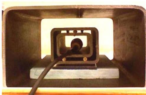
*Naïve* cells must be kept in a low 60-Hz MF environment, as laboratory and incubator fields are too high. Inside a low-field ( $0.4 \mu\text{T}$  average) incubator, Forma 3310, shielding is provided by three cylindrical layers of 6.3 mm thick structural steel. The three shields have outside dimensions  $15.2 \times 25.4 \times 36$ ,  $7.6 \times 10.2 \times 20$ , and  $5.1 \times 7.6 \times 20$  cm (Fig. 2.3).
