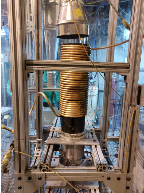
Figure 7.2: Burner With Copper Coil Wrapped for Heat Extraction Experiment
