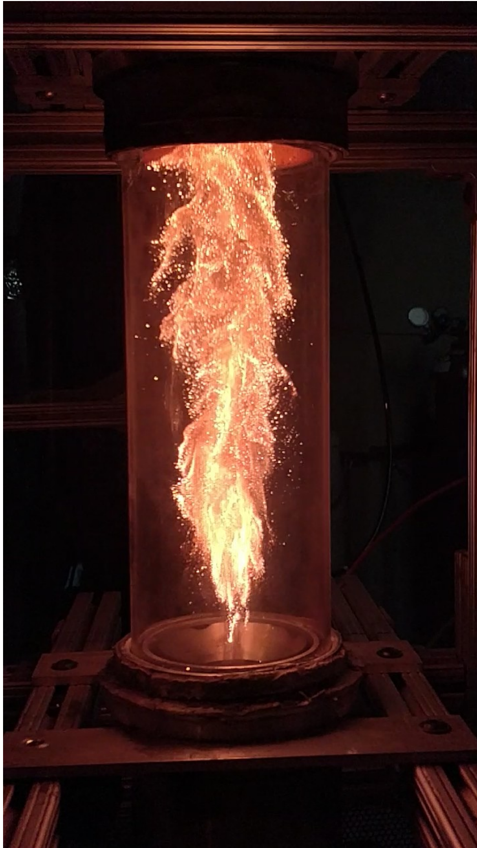
Figure 5.5: Self-sustained Turbulent Iron Burner Flame
