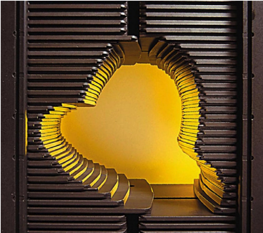
Figure 1.3: Picture of the 120 Millennium multileaf collimator from Varian®. The rounded leaf ends can be seen. From Bortfeld (2006).
