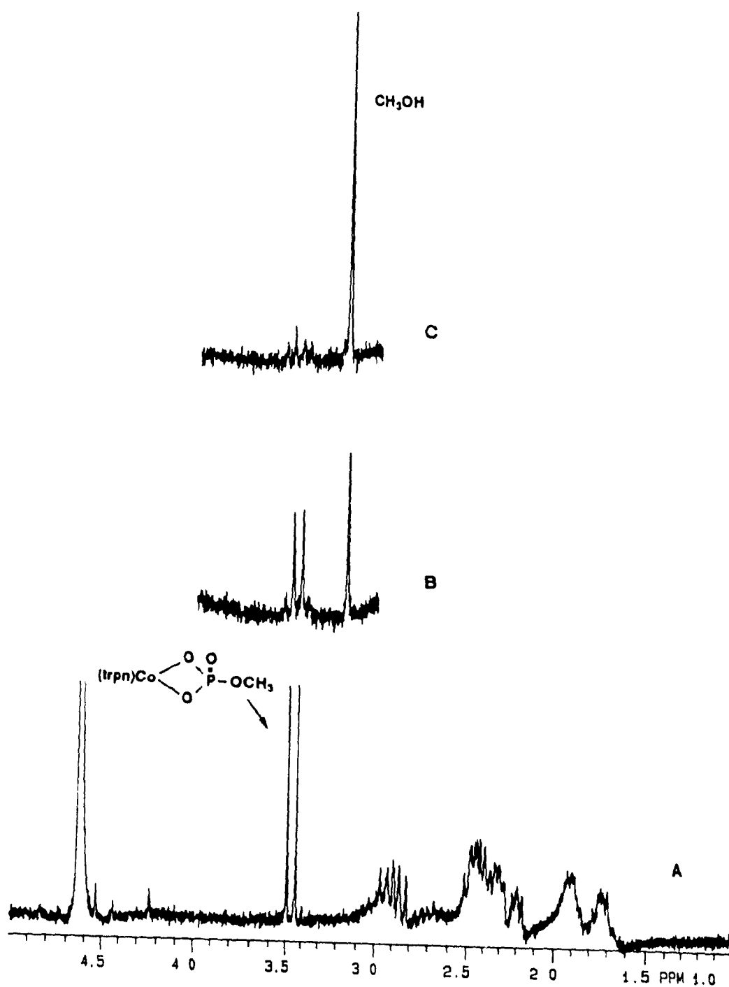
Figure 2.8 ^1\text{H} NMR spectra of methyl phosphate (5 mM) in \text{D}_2\text{O} after adding [\text{Co}(\text{trpn})(\text{OH}_2)_2]^{3+} (5 mM) and [\text{Cu}(\text{dpa})(\text{OH}_2)_2]^{2+} (5 mM), pD 7, 40 ^\circ\text{C} . Elapsed time A) 0 hr, B) 70 hrs, C) 214 hrs
