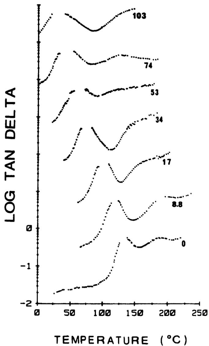
Figure 2.4. Loss tangent curves for the ionomers of Figure 2.2. Each curve is shifted up by an order of magnitude with respect to the previous one, for improved clarity.
