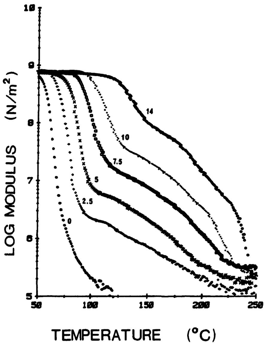
Figure 5.1. Dynamic storage modulus curves (1 Hz) for the C<sub>11</sub> ether series; ion contents vary from 0 to 14 mole%, as indicated.
