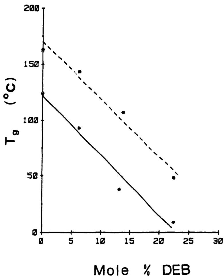
Figure 3.3. Matrix (—) and cluster (----) glass transition temperatures of PS-0.05MAA-Na ionomers plasticized with diethylbenzene, as estimated from Ref. 21.
