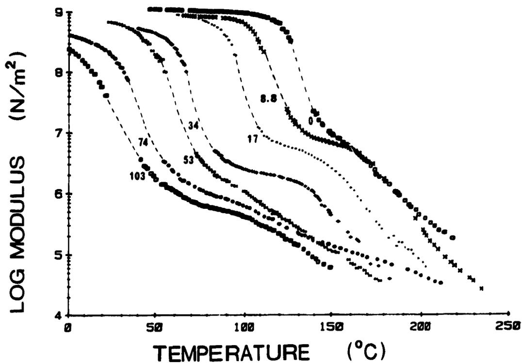
Figure 2.2. Storage modulus curves for the PS-0.07MAA-Na system alkylated with 1-decene. The curves are identified by the mole % of styrene rings with alkyl chains grafted on them.
