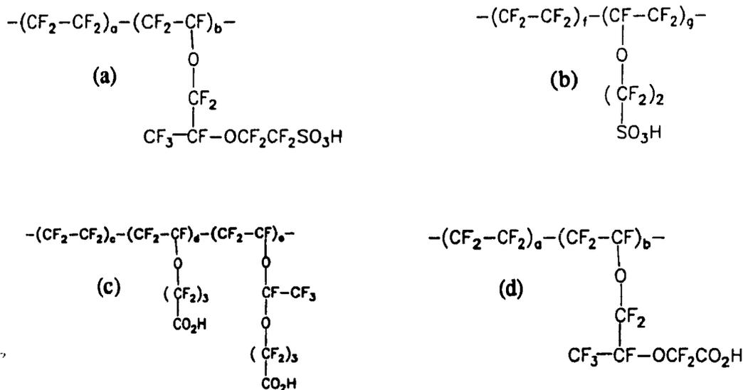
Figure 1.1. Examples of some commonly available perfluorinated membrane materials: (a) a sulfonated Nafion<sup>50</sup>, (b) Dow Chemical product<sup>51</sup>, (c) a carboxylated Flemion<sup>52</sup>, (d) Asahi Chemical product<sup>53</sup>.
