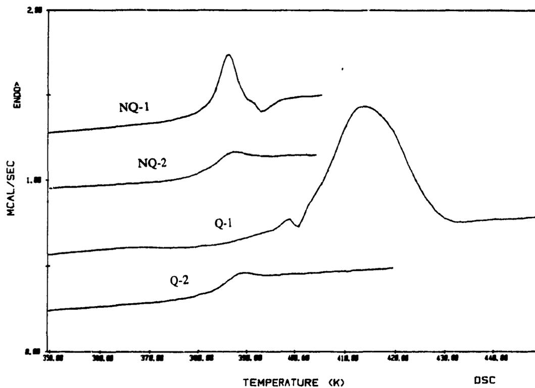
Figure B.1. Comparison of the first (1) and second (2) DSC scans obtained for PS-0.10 DMAS copolymers nonquaternized (NQ) and quaternized with methyl iodide (Q).
