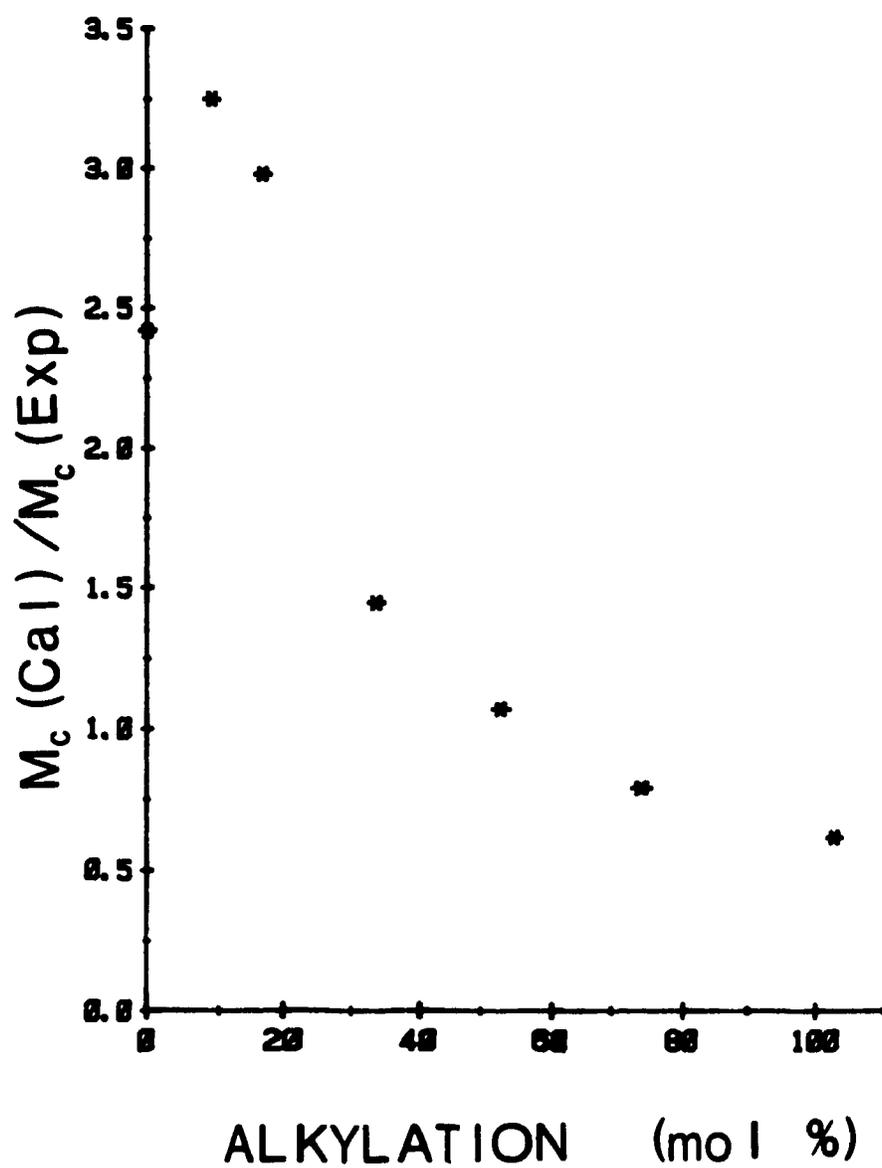
Figure 2.6. Extent of aggregation observed in the alkylated ionomers expressed as the ratio of calculated  $M_c$  for multiplet-type interactions to experimental  $M_c$ .
