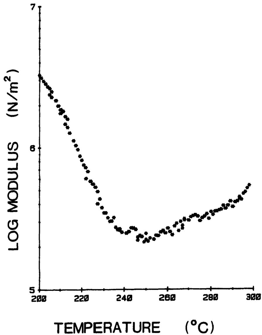
Figure 5.4. Storage modulus increase of the  $C_{11}$  ether 10% Na sample in the 200-300  $^{\circ}C$  range.
