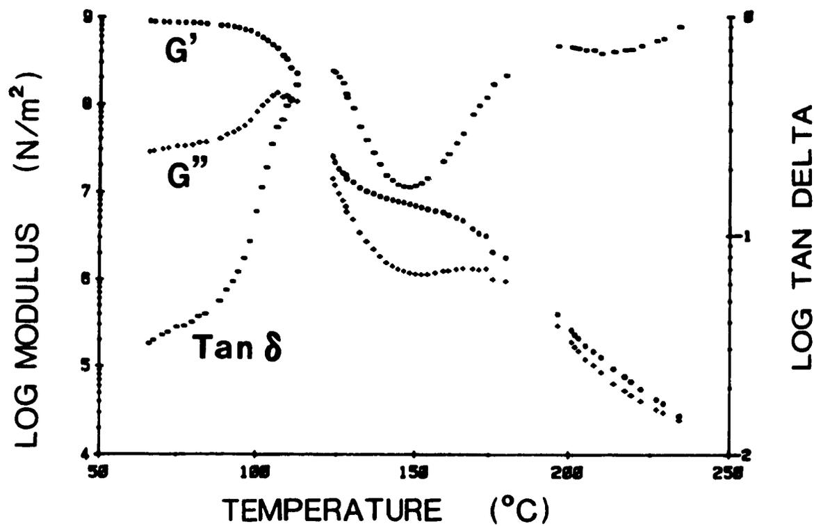
Figure 2.7. Original torsion pendulum curve for the PS-0.088Dec-0.07MAA-Na sample used as an example for the numerical data analysis.
