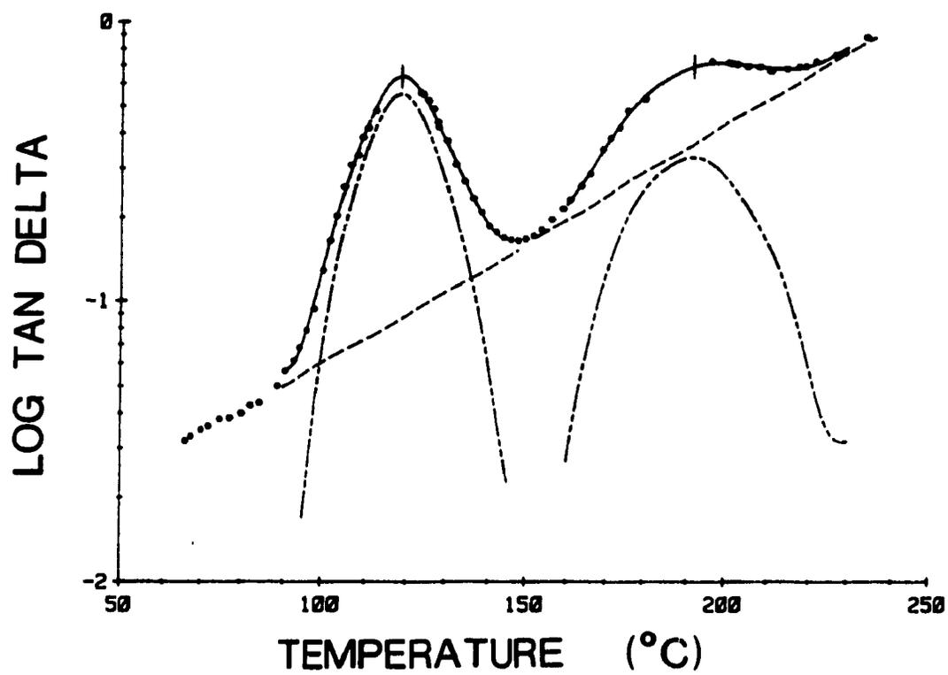
Figure 2.8. Curve fitting and baseline subtraction for the  $\tan \delta$  curve of Figure 2.7.
