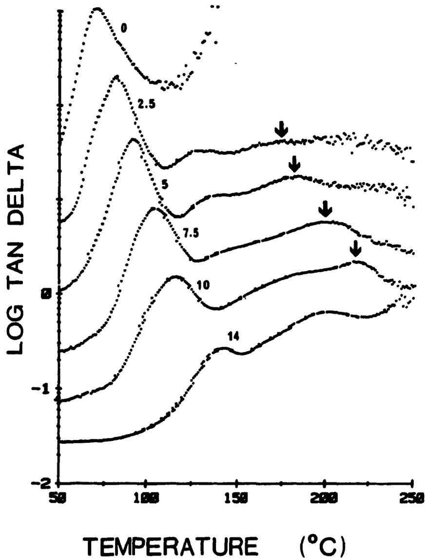
Figure 5.2. Loss tangent curves (1 Hz) for the ionomers of Figure 5.1. The scale indicated is correct for the bottom curve; each successive curve is shifted up by one half order of magnitude with respect to the previous one, for improved clarity.
