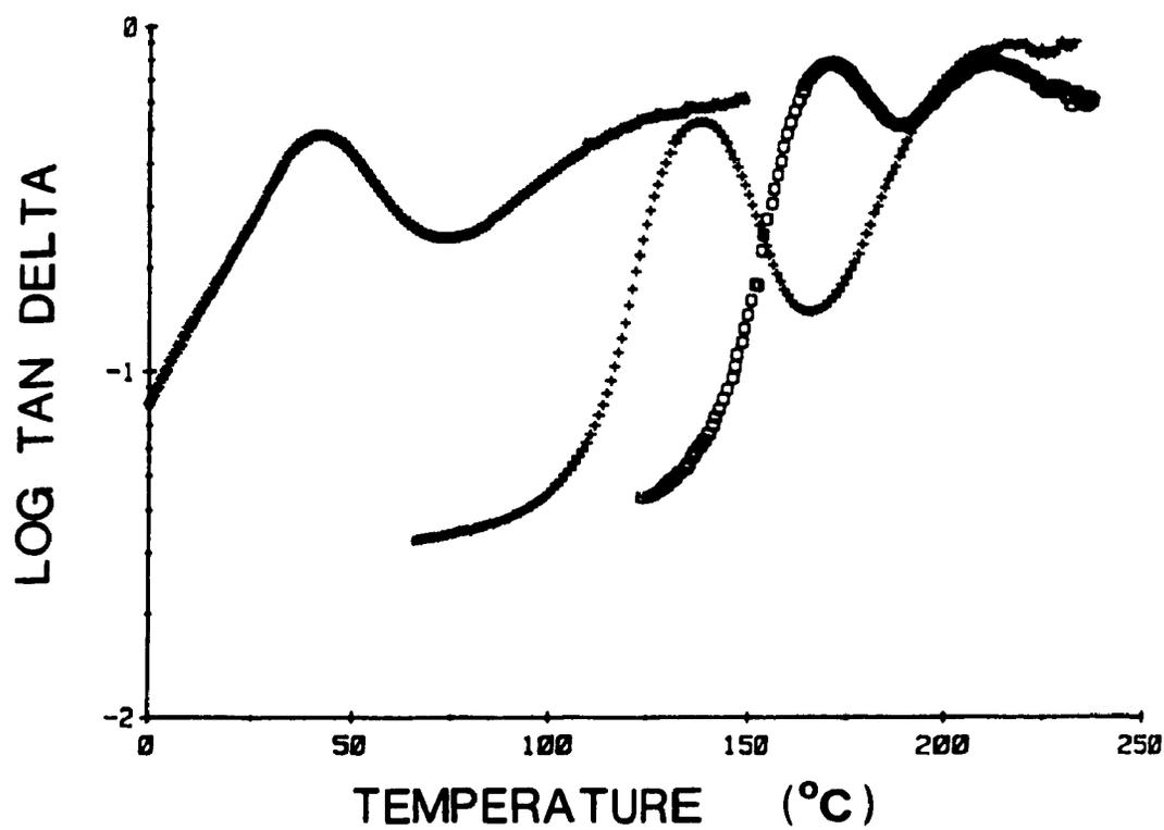
Figure 3.2. Dynamic loss tangent curves of + PS-0.07MAA-Na, O PS-0.07MAA-Na 32% nitrated, \* PS-0.07MAA-Na plasticized with 25% mol/mol (30% w/w) nitrobenzene.
