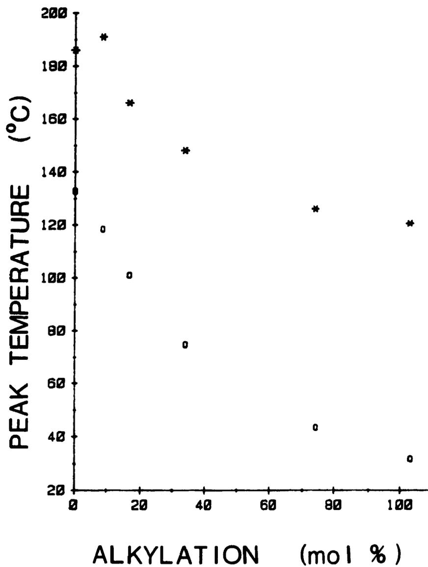
Figure 2.5. Peak positions of the loss tangent maxima associated with the matrix (O) and ion-rich domains (\*) for the alkylated PS-0.07MAA-Na ionomers.
