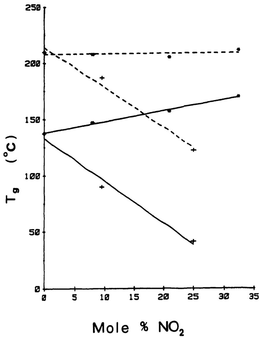
Figure 3.4. Peak positions of the dynamic loss tangent maxima in PS-0.07MAA-Na nitrated (\*) and plasticized with nitrobenzene (+) for the matrix (—) and ion-rich domains (-----).
