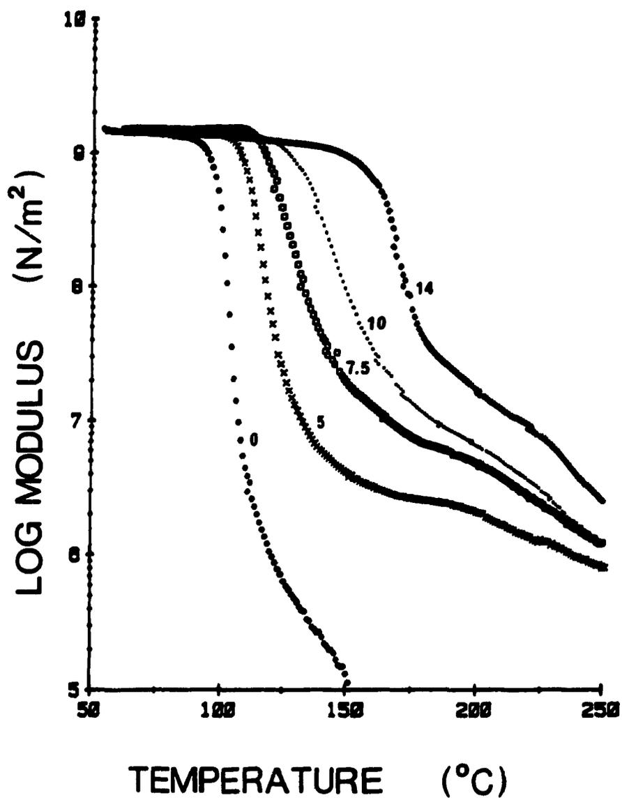
Figure 5.3. Dynamic storage modulus curves (1 Hz) for the C<sub>2</sub> ether series; ion contents (mole%) are as indicated.
