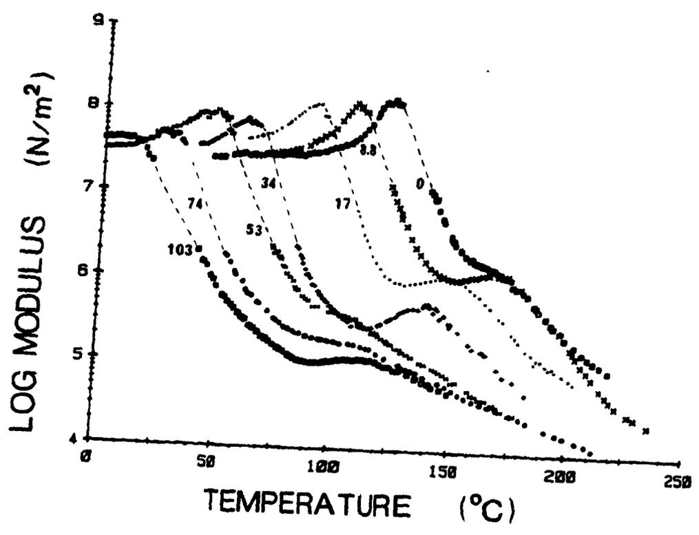
Figure 2.3. Loss modulus curves for the alkylated PS-0.07MAA-Na ionomers.
