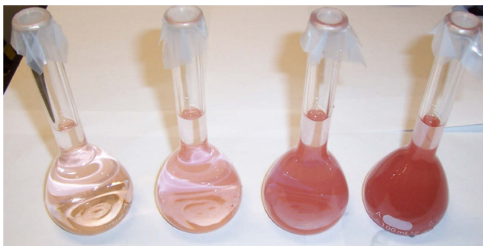
Figure 43 – Color variation of solutions of different turbidity following 20x dilution (from left to right 50, 100, 250 and 500 mg/L initial selenium concentration)
