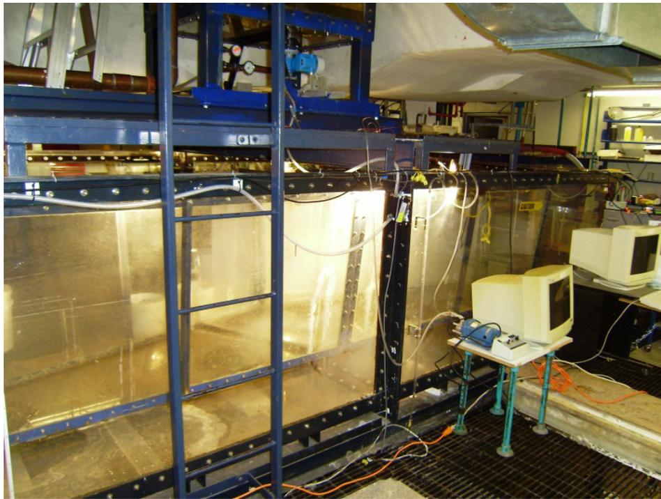
Figure 3.1 – A water model of a full scale 12 tonne delta shaped water model tundish at McGill Metals Processing Centre
