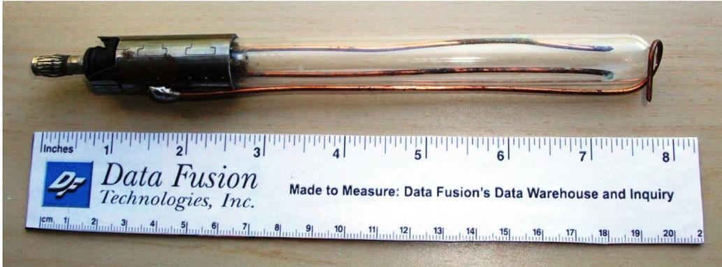
Figure 2.2 – Image of the detector probe designed by Heraeus Electro-Nite for APS II
