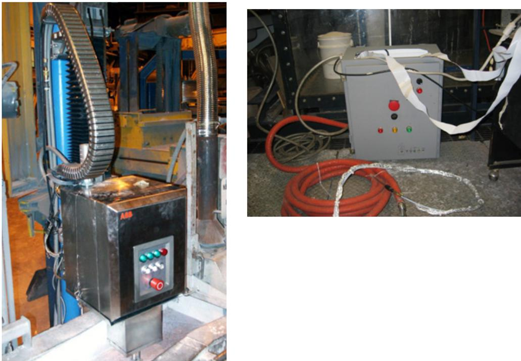
Figure 1.25 - a) LiMCA CM manufactured by ABB for molten aluminum,
