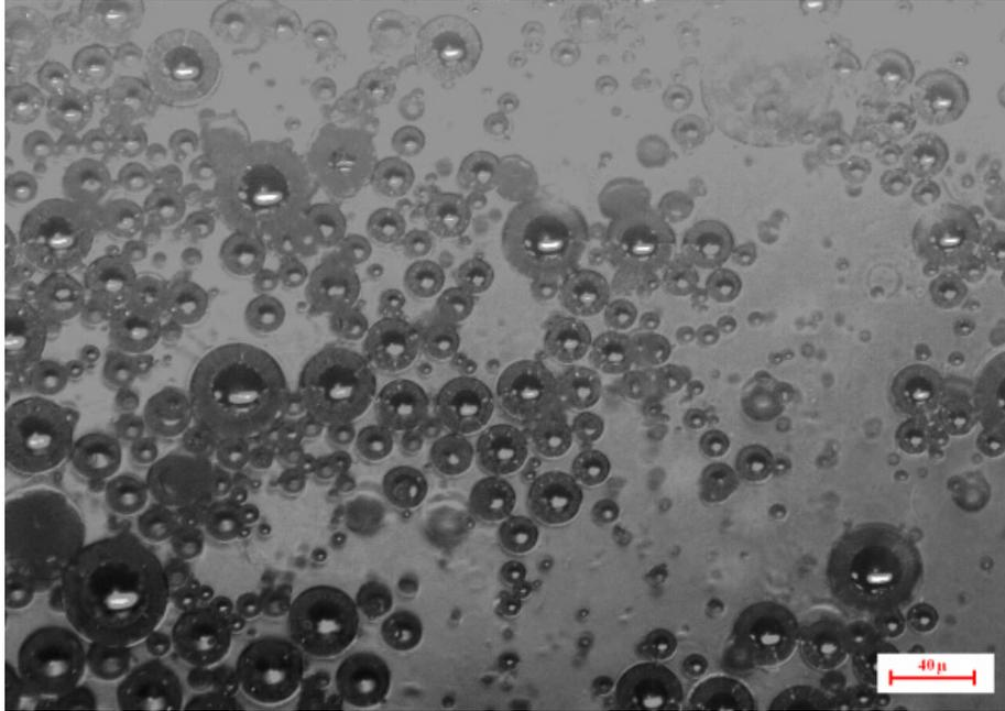
Figure 3.8 – Microscopic view of the hollow glass microspheres used to simulate inclusions
