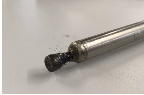
Fig. 35: Threaded device used to pack fuel pellets axially (Ferrari et al., 2019).
