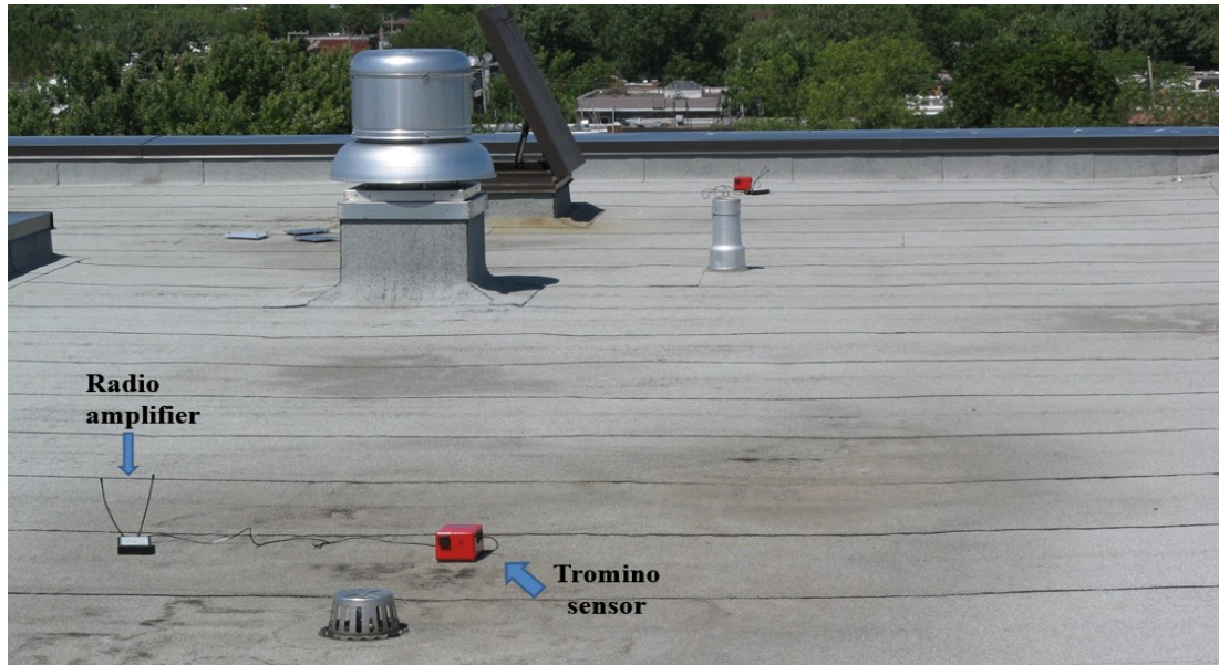
Figure 2.3 Wireless Tromino sensor and radio amplifier used for AVT
