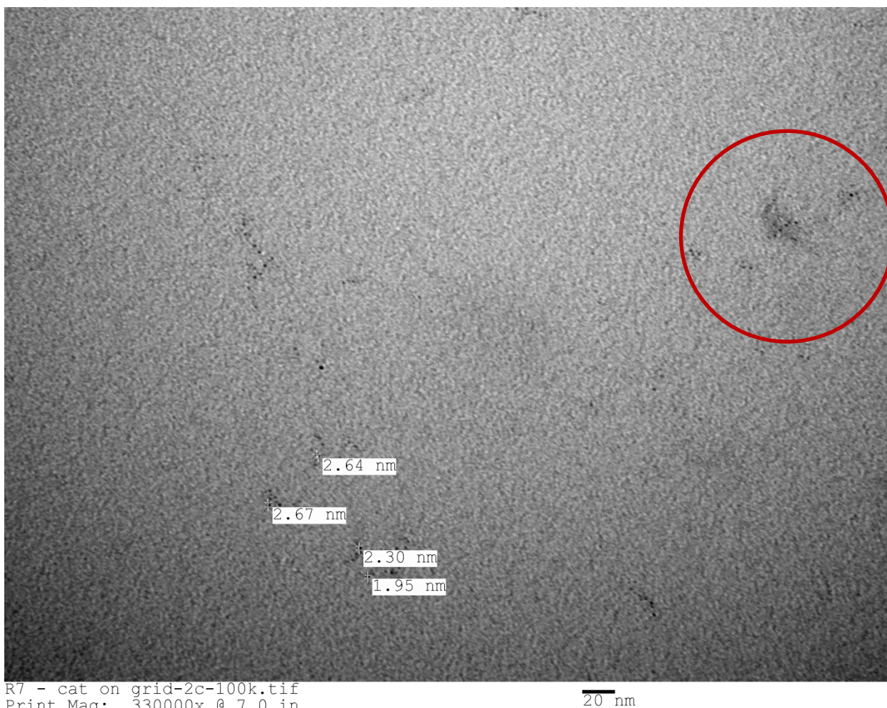
Figure 5.13 TEM image of Catechin on grid for CAT+AuNP Nanofluid
