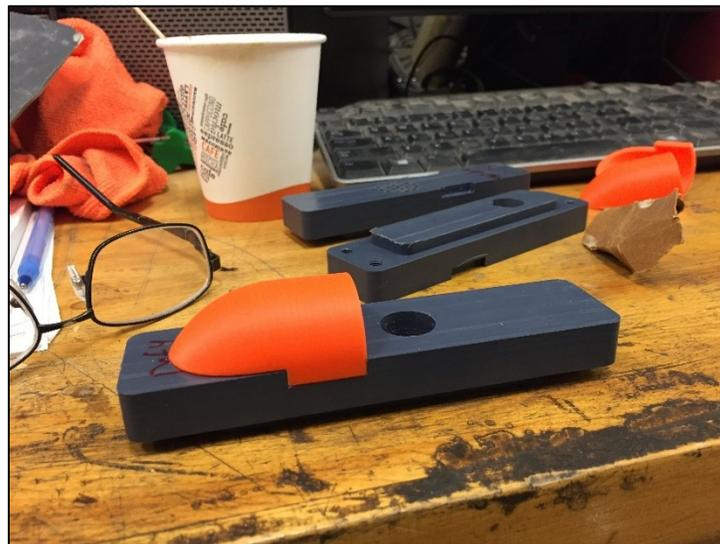
**Figure 3-12: Deflector attached to PVC Strip ( $H = 16.5\text{mm}$ ,  $L/H = 1$ )**
