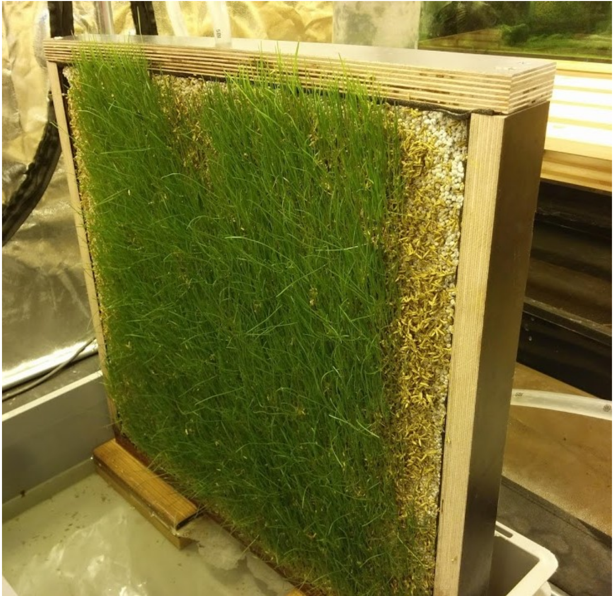
Figure 3.2.5: Vertically grown grass on permeable alkali activated porous concrete.
