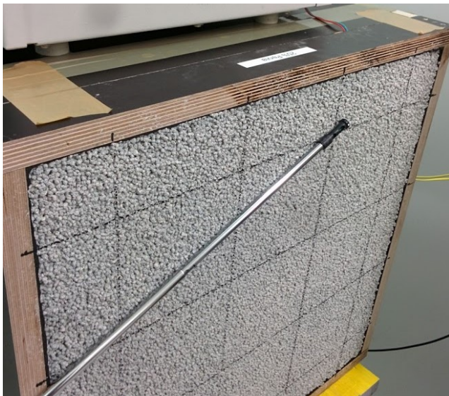
Figure 3.2.3: Experimental setups (wind tunnels) used for measuring permeability. Top and bottom left: Experimental setup for testing samples 1 - 6. Average air flow through samples was calculated by area averaging the results taken at each point where lines crossed (bottom left). Top right: Sensor placement for top left experimental setup. The array of thermocouples (top right) were located at 3.5, 9.75, 19.5, 35.5, 51.5, 61.0 and 67.2 cm from the bottom left along the diagonal line connecting the bottom left to the top right of the wind tunnel. Bottom right: Experimental setup for testing samples 12 and 13.
