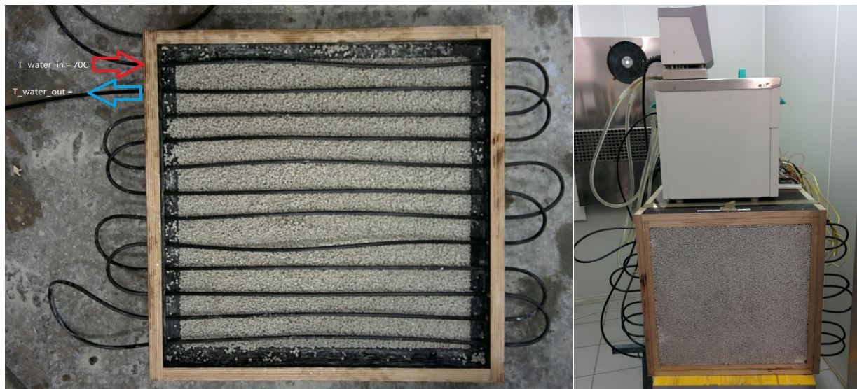
Figure 6.4.1: Porous concrete heat exchanger concept. Left: The center of the slab halfway through casting. Right: Experimental setup for heat exchanging slab.
