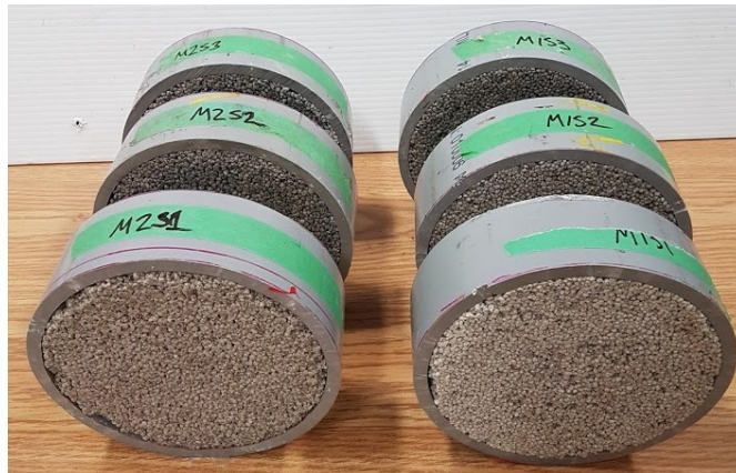
Figure 4.2.1: Mix design and visual appearance of porous concrete at varying water to binder ratio. Left: Mix design for two water to binder ratios (0.25: M1 and 0.35: M2). Right: Visual appearance of tested samples. The first two digits (M1 or M2) represent the mix and the second two (S1, S2 and S3) indicate unique individuals. Bernasconi is a quartz aggregate (Quarzsand, 2 – 3.2mm, Carlo Bernasconi AG, Berne, Switzerland).
