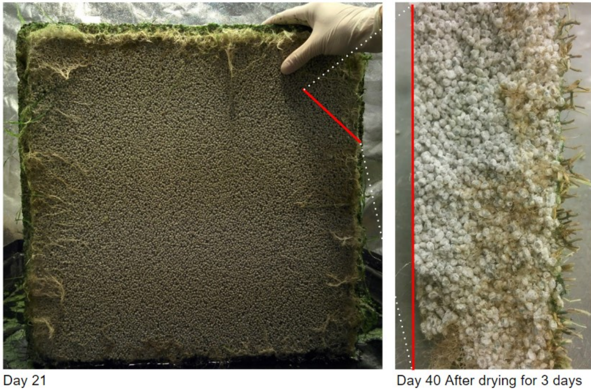
Figure 3.4.1: View from underneath slab and cross section of roots after drying.
