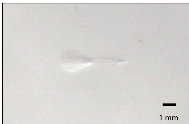
Figure 4-1. Gas check defect on a PVC film.
